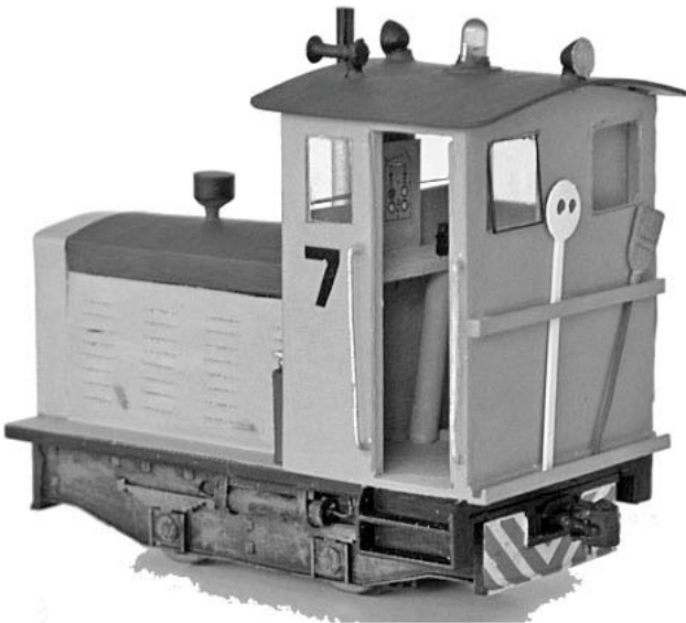
Comeng Model A inspired On30 4w DM locomotive, scratchbuilt styrene superstructure on a Boulder Valley resin chassis, power unit from a HO Bachmann 44 ton diesel and working Circuitron flashing light. Lynn Zelmer, model builder and photographer.
