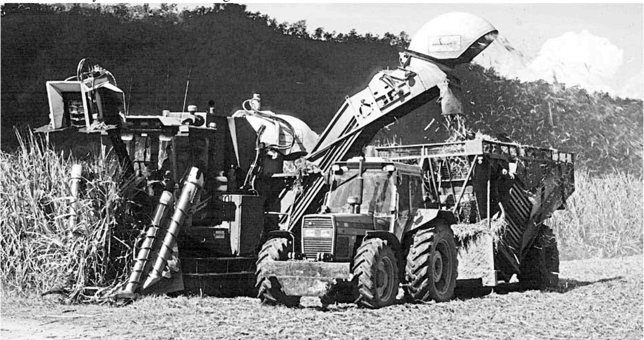
A tractor-hauled infield transporter being filled by an Austoft cane harvester. This type of transporter elevates and tips to fill cane bins on the nearby cane tramway. Other infield options include one or more cane bins on a tractor-hauled trailer or semi-trailer truck. Greg Stephenson, photographer.
