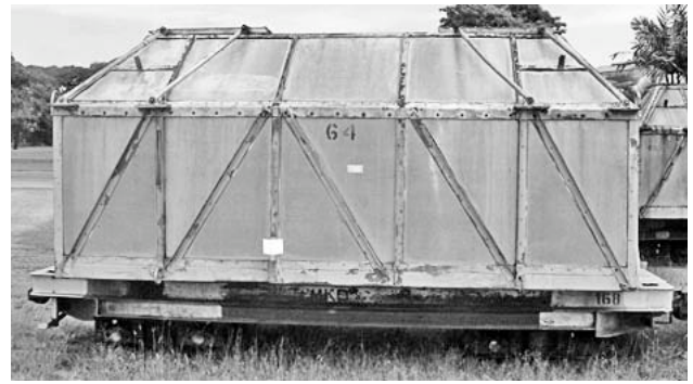
Herbert River Mills' (Victoria and Macknade) side dumping bulk sugar wagons, 2005. Brian McWilliam, photographer.
