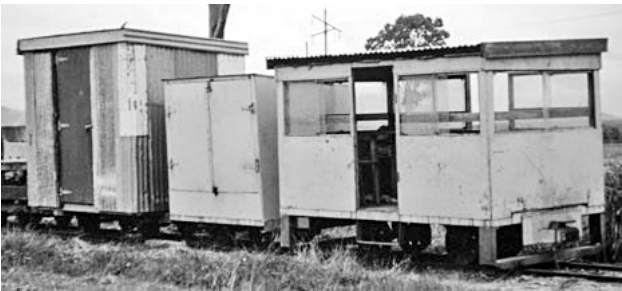
Marian Mill navy equipment [previous column], 1986. The far wagon is likely built on an old cane bin frame, the centre metal cabinet on an old wholeshtick truck. Greg Stephenson, photographer.
