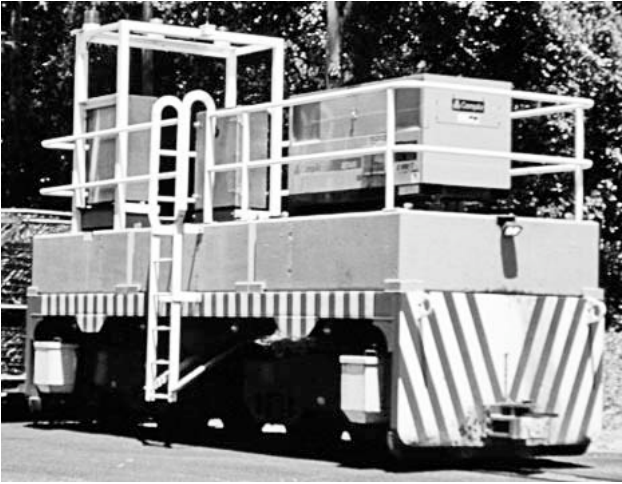
Mulgrave Mill bogie brake van. Since cane bins are unbraked some mills use a mid-train or end-of-train brake van, essentially a compressor, radio controls and a heavy braked frame. Greg Stephenson, photographer.
