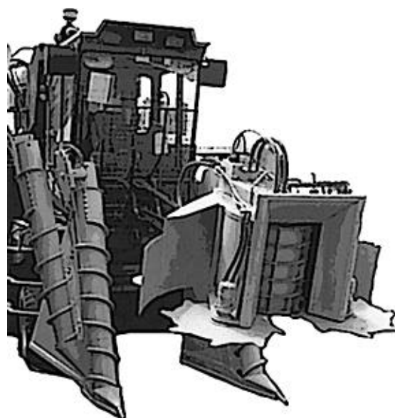
The dual cutters on this harvester (above) raise up and down to cut the leafy tops off the cane. The roller mechanism guides the cane into the billet cutters. Leaves and other trash are blown out the back while the billets are dumped into a bin or in-field transporter moving along beside the harvester.
