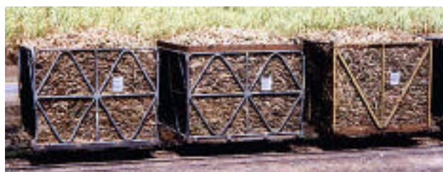
Three different four ton bins: now operating together they originally came from different mills. The boards on the top of the middle bin extend its capacity. Some bins had one solid side to make dumping easier.
