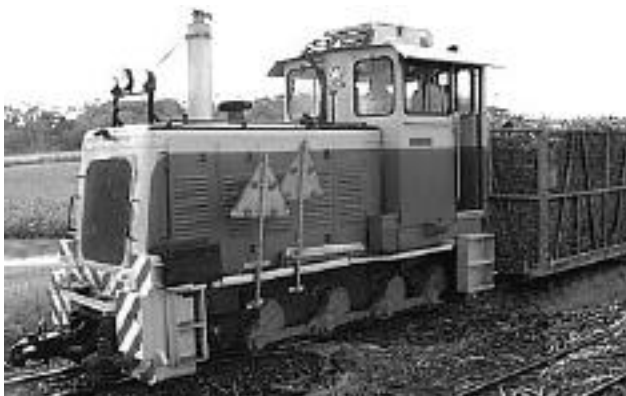
St Helens (Farleigh Mill, Mackay), an 0-6-0. Note the end-of-rake markers and wooden wheel chocks on the side of the loco, plus the air conditioner and flashing lights on the roof.
