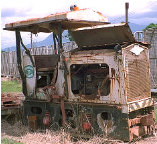
First generation Malcolm Moore locomotive, similar to those at the Australian Narrow Gauge Railway Museum (Woodford) and most recently used for maintenance work. Note the yellow flashing safety light on the roof.
