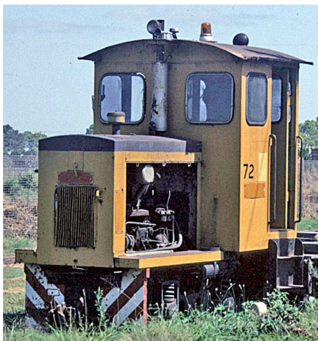
The loco is now numbered 72 and sports its most recent colour scheme in this 1999 photo by Greg Stephenson. Cane locos often received significant modifications over time, a change in paint scheme being a relatively minor alteration. The removal of the ventilated hood cover on at least one side suggests that the loco runs too hot, a common occurrence with older locos of any size in tropical conditions.
