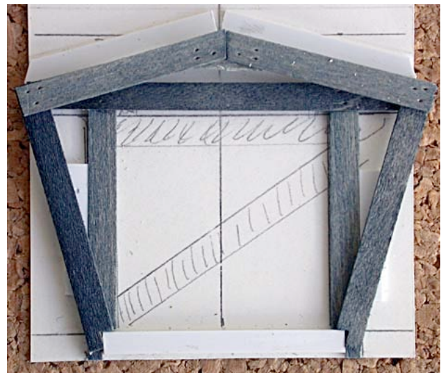
Simple jig 3 with superstructure timbers being combined to form internal uprights and roof supports. Nut/bolt/washer castings will be applied to simulate bolting together.
