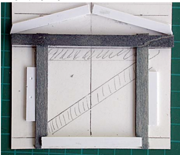
Simple jig 1 with 2 x 8 timbers for internal superstructure being superglued. Note nail holes where timbers join.
