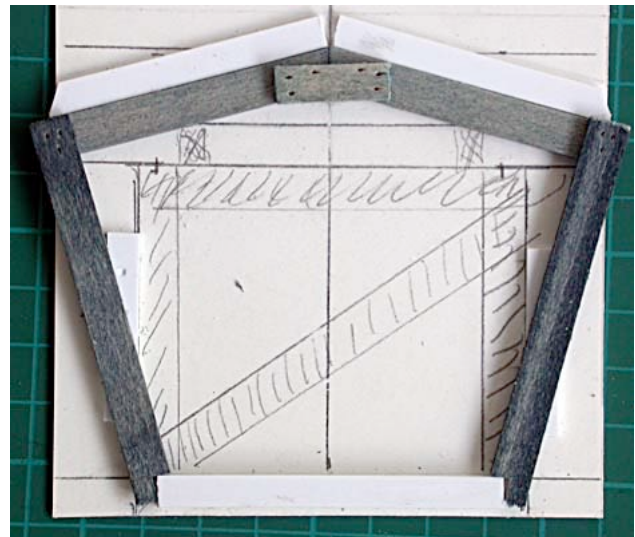
Simple jig 2 with roof support timbers being superglued. Nail 'holes' have been added with a sharp pick and later will be highlighted with weathering.
