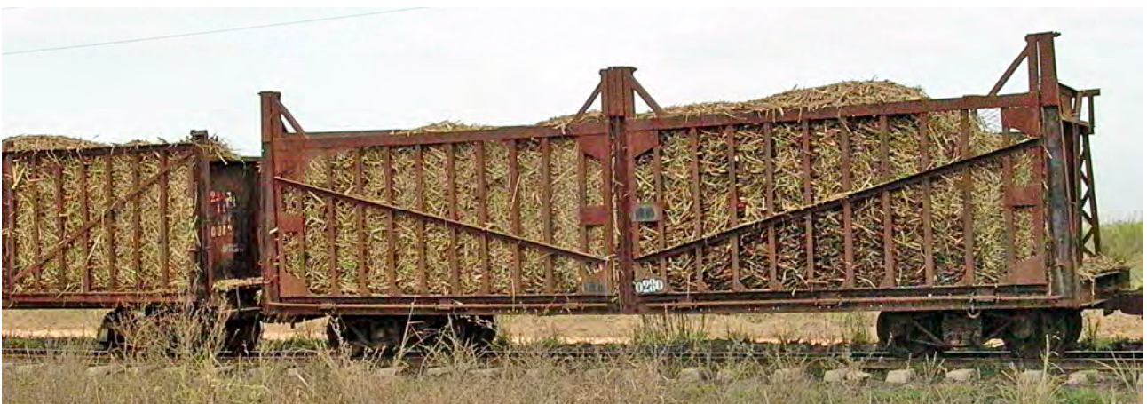
Gregorio Arlee Manalich Mill, Cuba: 2 ft 6 inch gauge sugar cane wagon, February 2003. Note how much longer this wagon looks than the models immediately above, however a wagon this long might not get around On30 curves. Claus Kleinhapl photographer.
