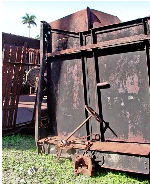
Pepito Tey Mill, Cuba: damaged sugar cane wagon (end view), February 2003. Note solid metal end and side release mechanism. Claus Kleinhapl photographer.
