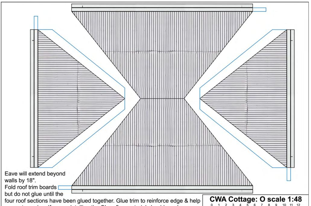
prevent warping. If super-detailing the CI roofing material should overhang roof (ie trim boards) by 3" on all 4 sides.
