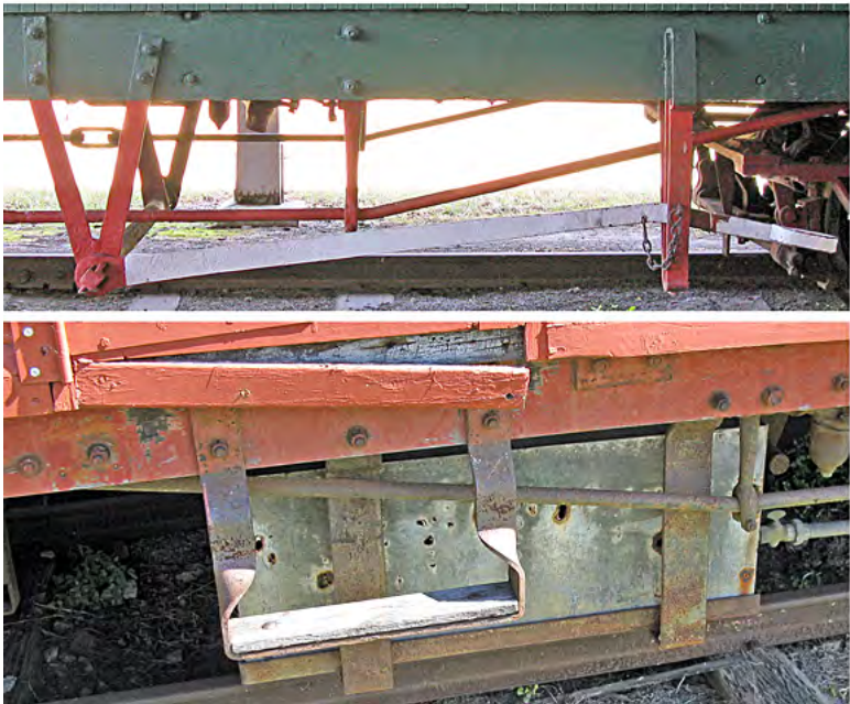
Standard 32' camp wagon being restored at Woodford (CW154), and QR 2 Man Camp Wagon (class CW) drawing adapted from QR wagon drawing 304 (Ipswich) of 1971. Windows, doors and other details varied with 2, 3 and 4 man capacity and which workshop constructed the wagon.
