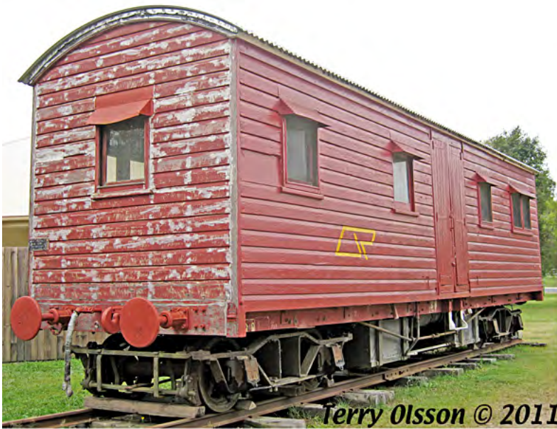
Standard 32' camp wagon being restored at Woodford (CW154), and QR 2 Man Camp Wagon (class CW) drawing adapted from QR wagon drawing 304 (Ipswich) of 1971. Windows, doors and other details varied with 2, 3 and 4 man capacity and which workshop constructed the wagon.
