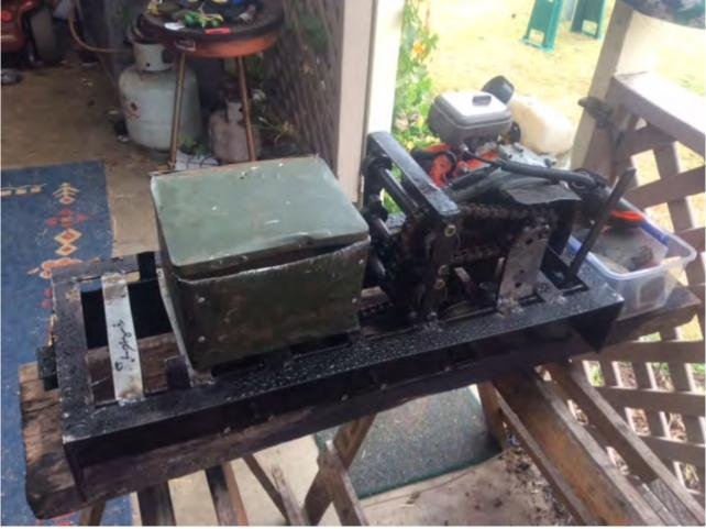
The recently overhauled drivetrain and retrofitted "cupcake tray" for ballast weight. Lady T's powerplant is a ~25cc whipper snipper engine, with a 10:18, 10:18, 10:16 gearing reduction in the drivetrain via a centrifugal clutch.
