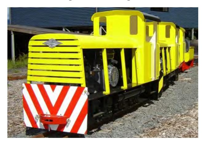
The third of three locos built to this design at the "Boulder Creek Loco Works". The loco dimensions are 1590mm buffer beam to buffer beam (1750mm overall), 554mm in width, and 970mm rail head to roof top. Total weight is 338 kg's.
