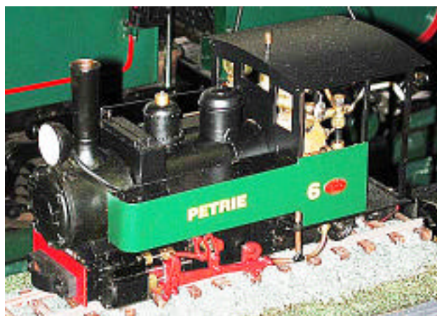
Steve Malone's coal-fired 16mm scale (32 mm gauge) Fowler model. Not shown: a garden railway with a small diesel pulling whole stick trucks and a small HOn30 cane operation as part of a larger HO layout.
