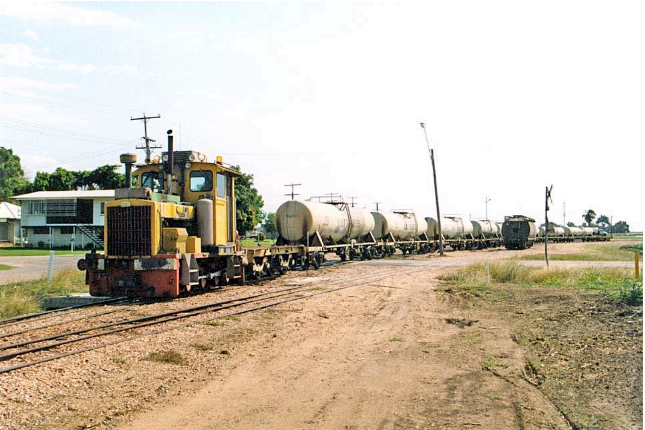
Kalamia Sugar Mill locomotive Airdmillan lifts a rake of QR Molasses wagons out of the exchange siding at Ayr. The wagons at each end of the train are match wagons.
