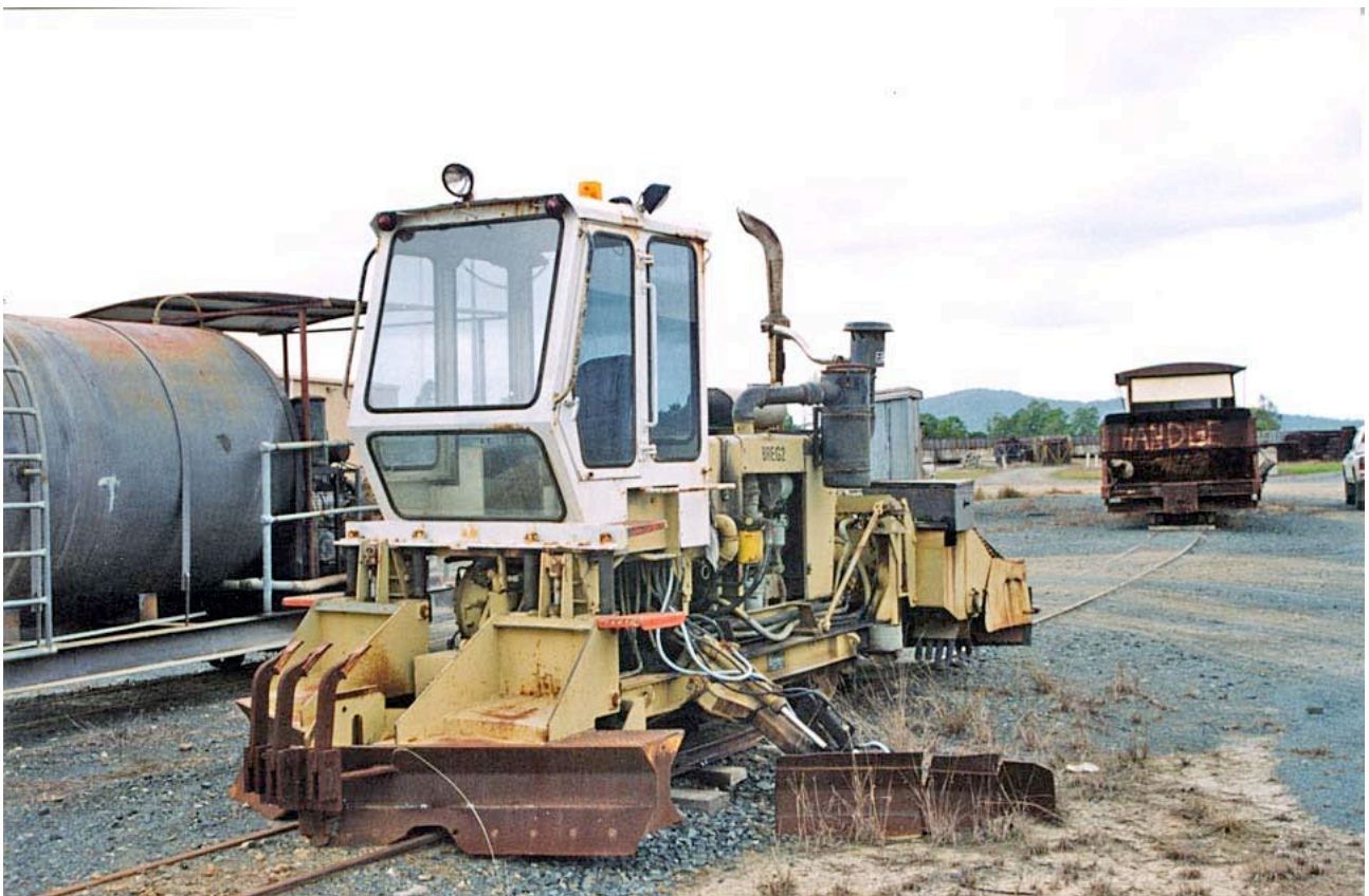
Canron ballast regulator, Marian Mill
