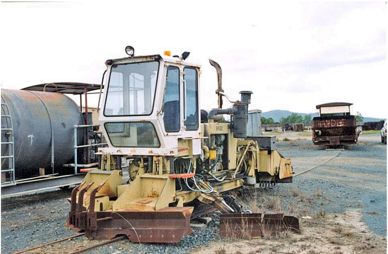
Canron ballast regulator, Marian Mill
