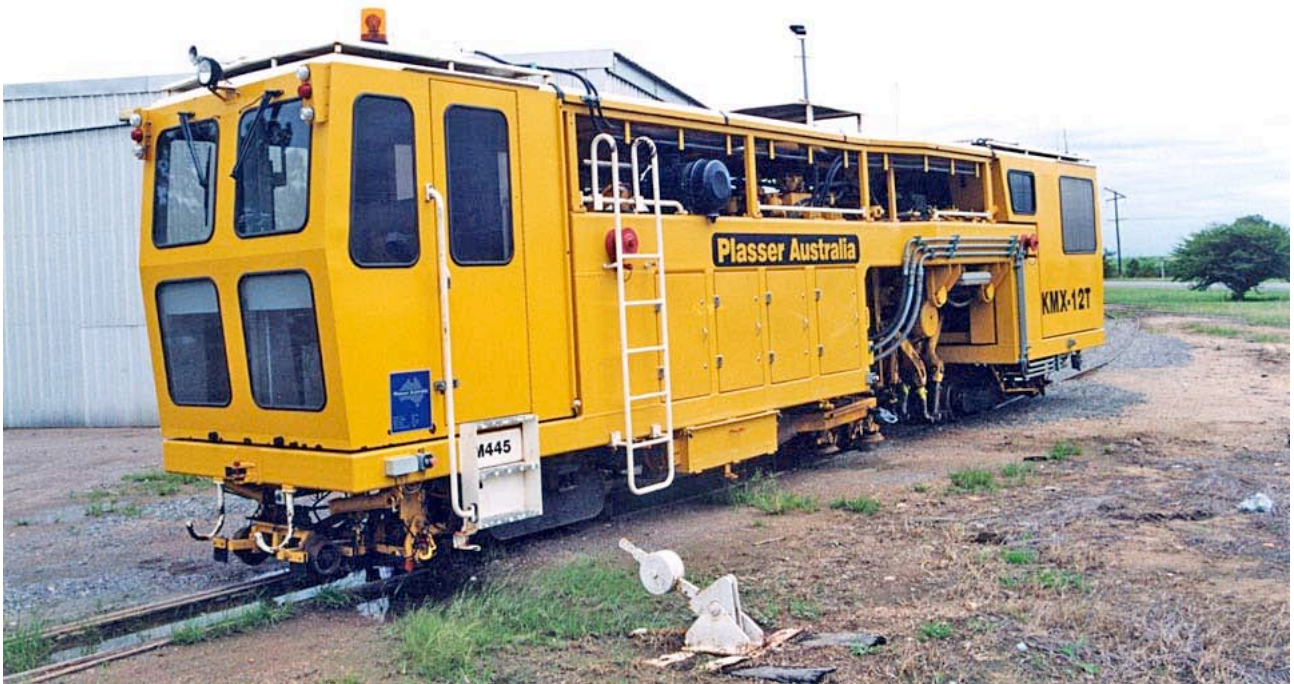
Plasser KMX-12T tamper liner, Victoria Mill
