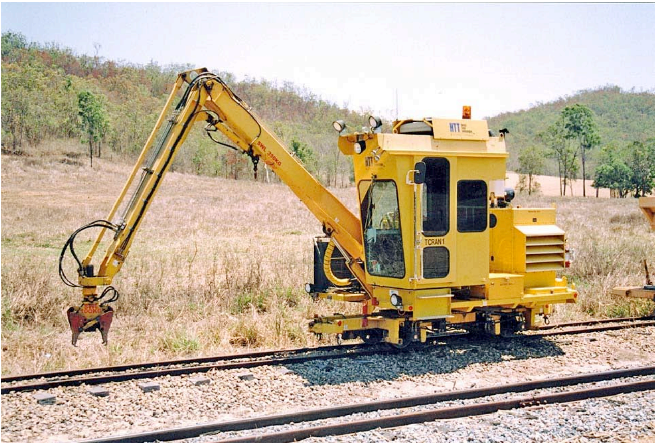
Harsco sleeper crane, Farleigh Mill
