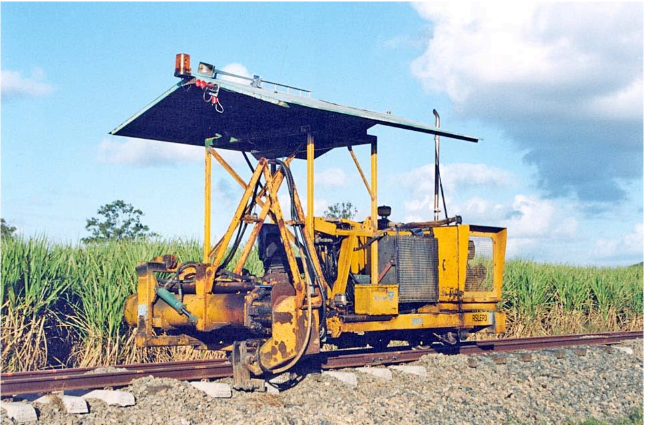
Fairmont Tamper sleeper replacer, Farleigh Mill
