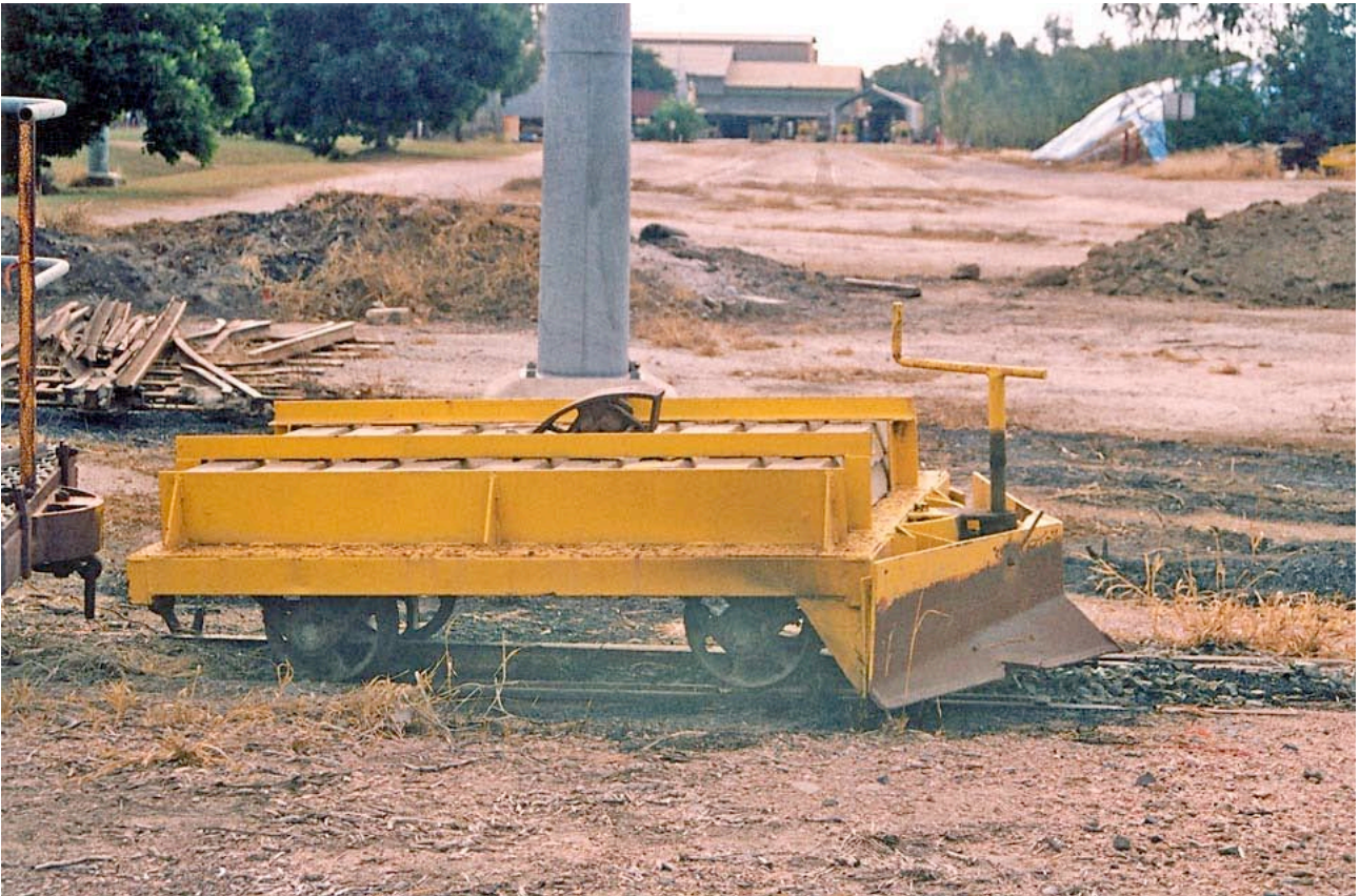
4 wheel ballast plow, Inkerman Mill
