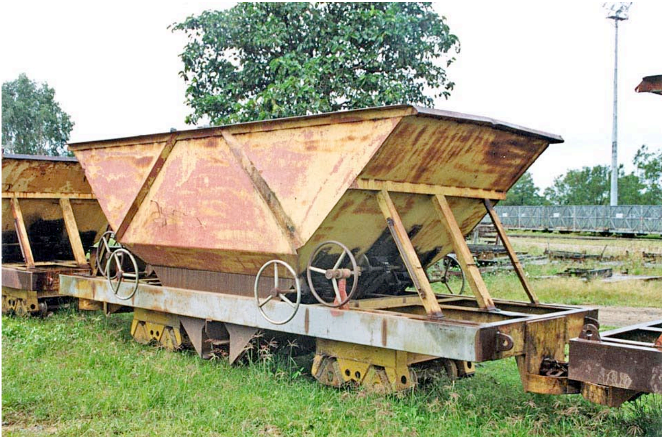
Bogie ballast hopper, Proserpine Mill
