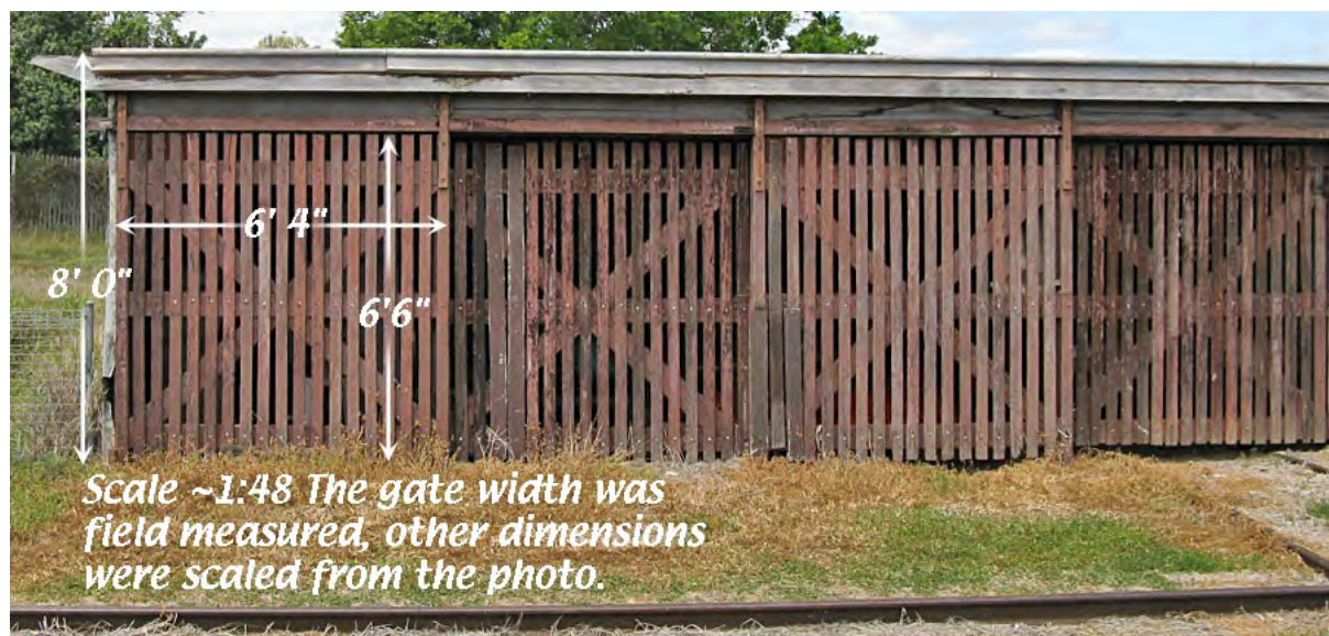
Basic dimensions for Mount Morgan fettler's shed.
