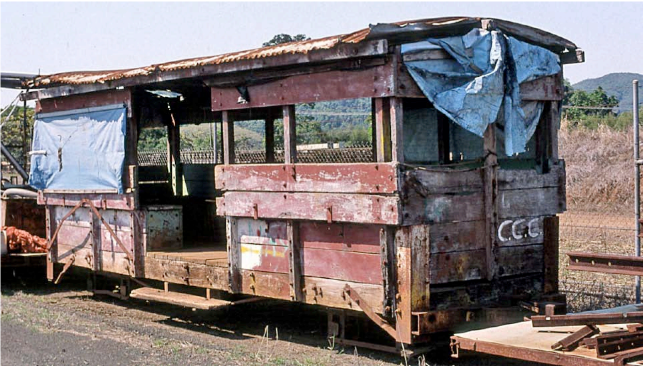
Navies wagon at South Johnstone Sugar Mill shows a typical Shire tramway type conversion of a bogie open wagon. Greg Stephenson, photographer.
