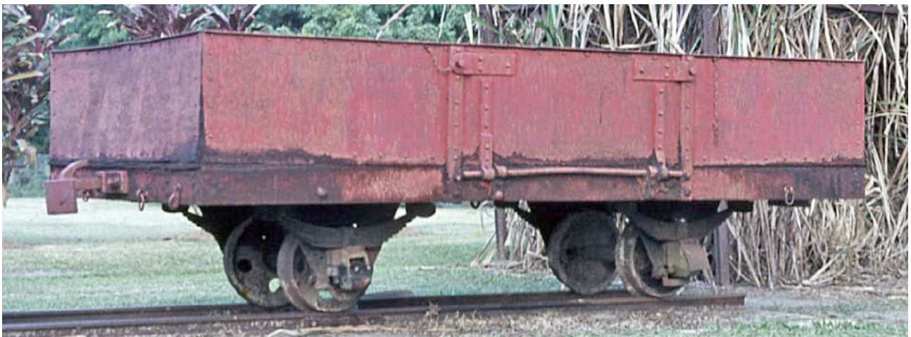
Douglas Shire Tramway steel 4 ton open wagon displayed at Mossman Mill. Greg Stephenson, photographer
