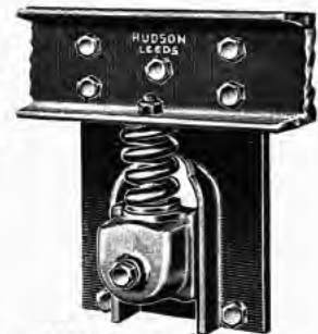
AXLEBOX with brass bush and spiral spring Code 36692
