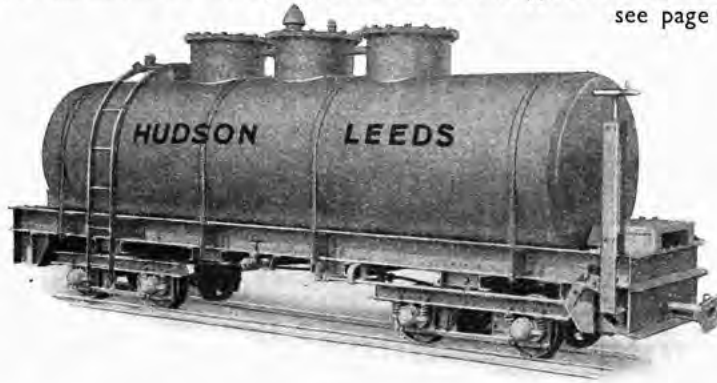
TANK WAGON for gasolene, 2500 gallons cap, mounted on bogies, with central spring buffers and screw brake Code 36597
