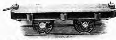
FLAT CAR steel platform, stanchion pockets and couplings Code 36580
