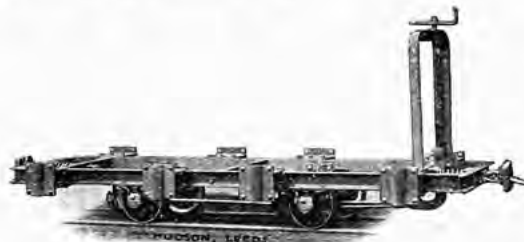
FLAT CAR with stanchion pockets, screw brake, spring buffers Code 36591
