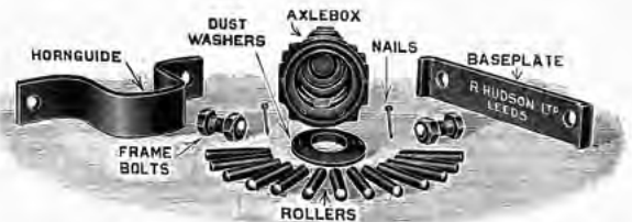
OUTSIDE SWIVEL TYPE BEARING DISMANTLED Code 36684
