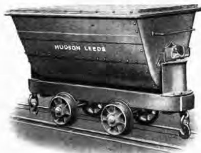
HEAVY TRUCK with rail top hoop and swivelling drawbars Code 36497
