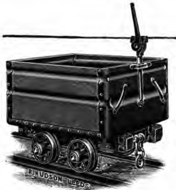
ENDLESS WIRE ROPE OVER THE TUB with clip. Stops may be placed to release the clip at any desired point
