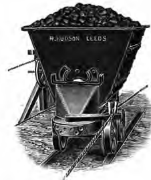
ENDLESS WIRE ROPE AT SIDE hauling Hudson side tip trucks of 20 cubic feet capacity, with side jockey
