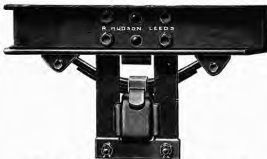
AXLEBOX with brass bush and laminated spring Code 36693
