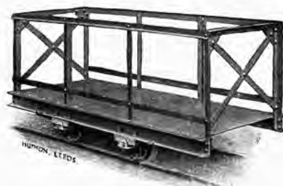
LIGHT BOX CAR steel platform, no buffers Code 36596
