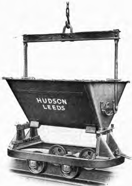
SIDE TIP WAGON with the body fitted with crane trunnions and feet. Can be tipped whilst the body is slung from the crane and also whilst on its underframe
