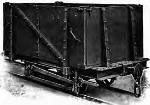
5 TON BOX CAR with sides and ends to lift out, timber body
