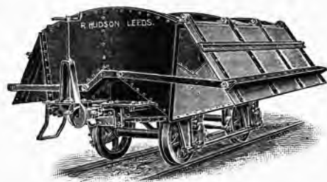
WAGON with side discharge doors, spring buffers and screw brake Code 36512
