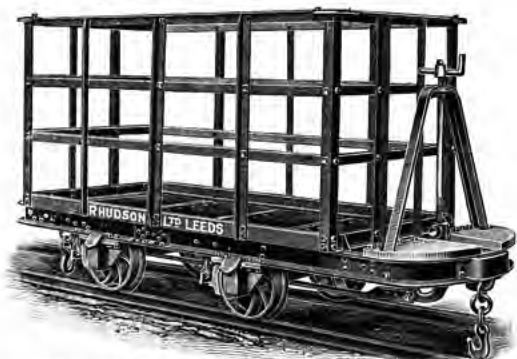
4 TON LIGHT CAR fixed ends and sides, steel platform Code 36561
