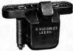
PLAIN AXLEBOX with anti-friction metal bush Code 36685
