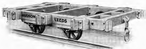
FLAT CAR steel platform, stanchion pockets, light couplings Code 36590
