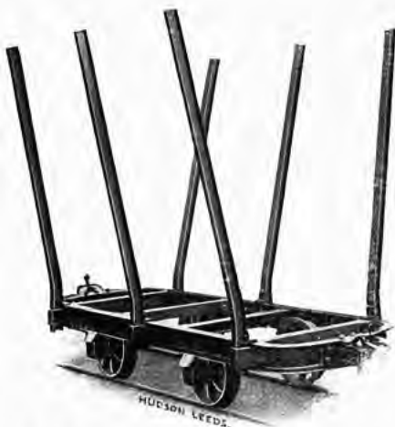
CAR FRAME with stanchions of light rails Code 36594
