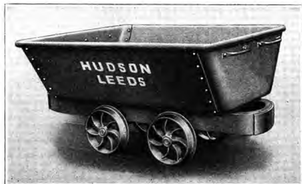
FLAT BOTTOMED TUB with tapered sides and ends Code 36550
