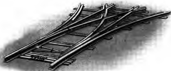
THREWAY TURNOUT on steel sleepers with kickover tongues
