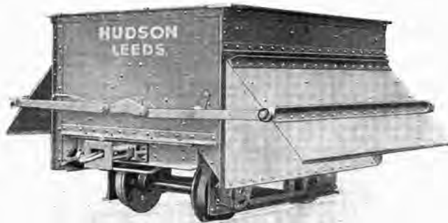
SMALL WAGON with side discharge doors, plain central buffers and drawgear Code 36509
