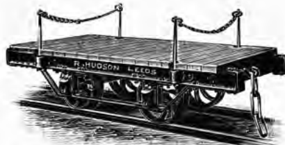
FLAT CAR heavy type, with timber platform, loose stanchions, side buffers Code 36588
