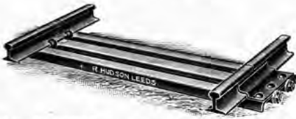
JOINT SLEEPER for clutchbolt type track for 10/20 lbs. rails. Dispenses with fishplates and bolts. Code 36114
