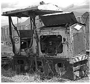
Malcolm Moore locomotive (above), similar to locomotives at the Woodford Narrow Gauge Museum railway and likely used for maintenance work. Note that even it has a yellow flashing light on the roof (not the original roof).
