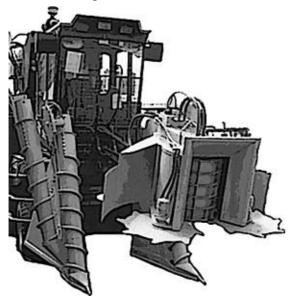
The dual cutters on this harvester (right above) raise up and down to cut the leafy tops off the cane. The roller mechanism guides the cane into the billet cutters. Leaves and other trash are blown out the back while the billets are dumped into a bin, usually moving along beside the harvester.
