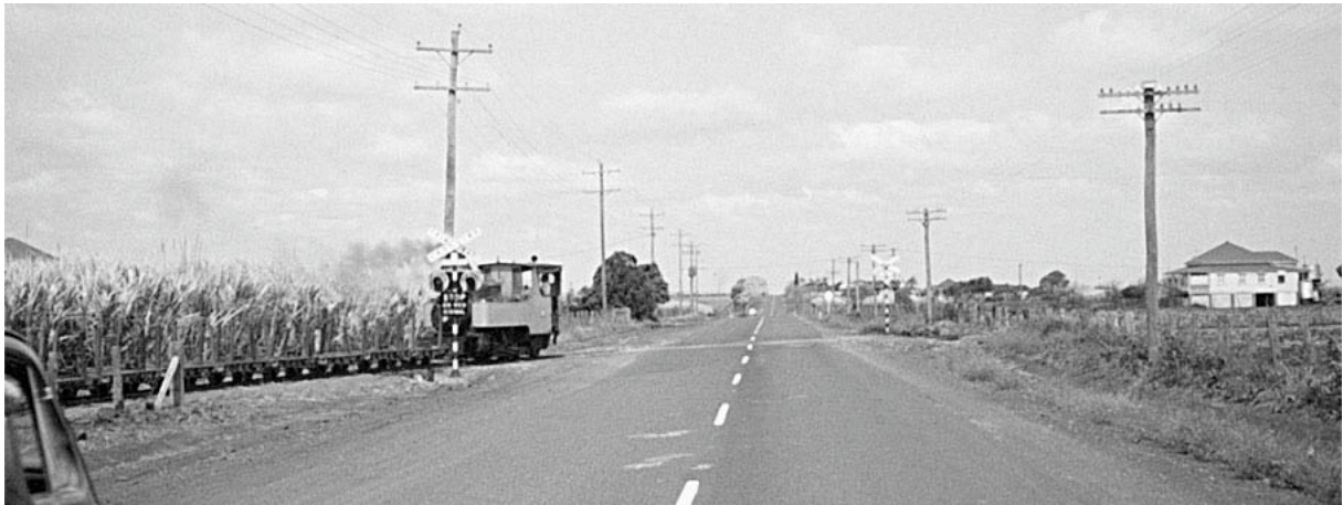
Brightly coloured steam locomotives were the norm in cane growing areas before dieselisation. Qunaba Mill 0-4-2T (Fowler, Leeds, No 20284, Millaquin Mill owners) crossing Burnett Heads Road with empty wholestick trucks, 24.9.63, John Browning Collection
