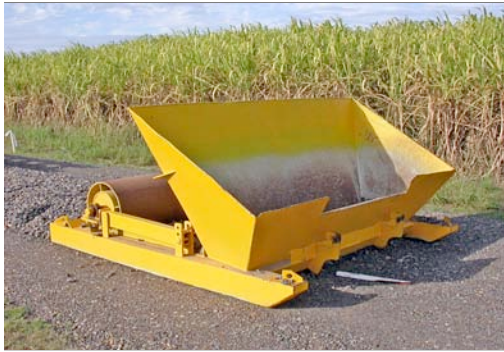
This ballast spreader also profiles the formation. Millaquin Mill, Bundaberg 2007
