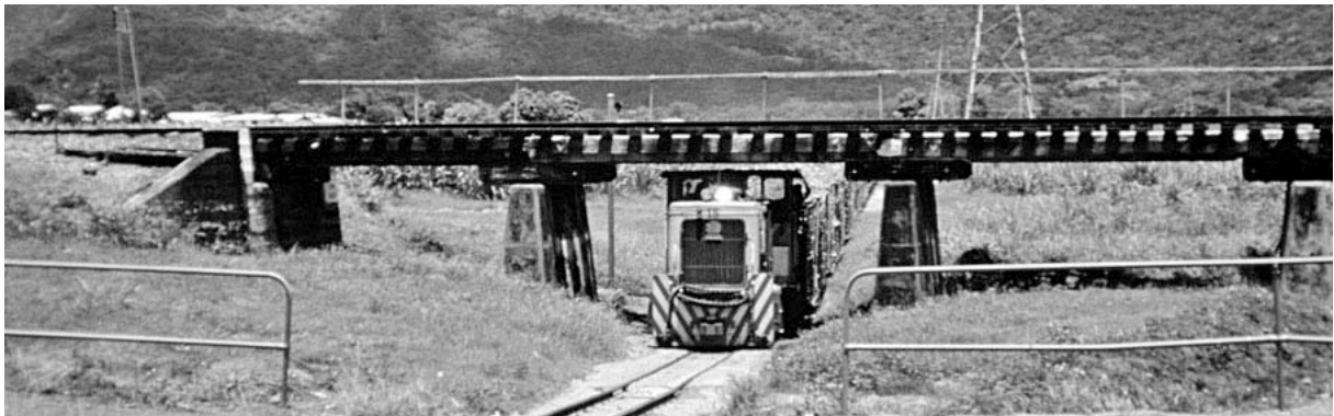
Some loco modifications arise from engineering changes, such as regauging or remotoring, some from repairs after accidents, and others from operational restrictions. Note the reduced height cab to fit under the QR overpass at Redlynch, Mulgrave Mill, 1995, Greg Stephenson, photographer
