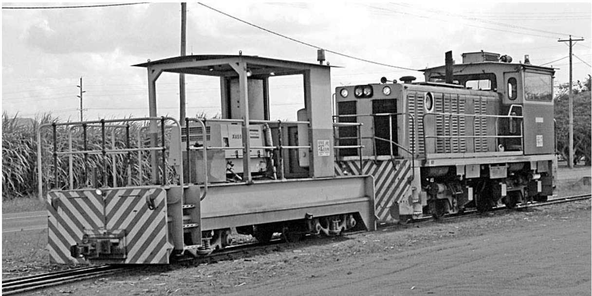
Regauged and rebuilt ex-mainline DH locomotives provide the power for faster, heavier trains. Mackay Sugar: rebuilt DH and bogie brake van, 2005, Jonathan Bayliss, photographer
