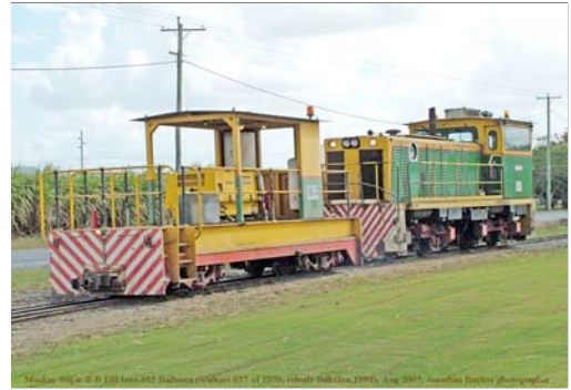
Mackay Sugar: rebuilt DH and bogie brake van, 2005, Jonathan Bayliss, photographer
