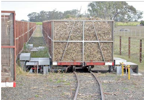
Strathdees, Millaquin Mill, Bundaberg 2007. Automatic bin mover
