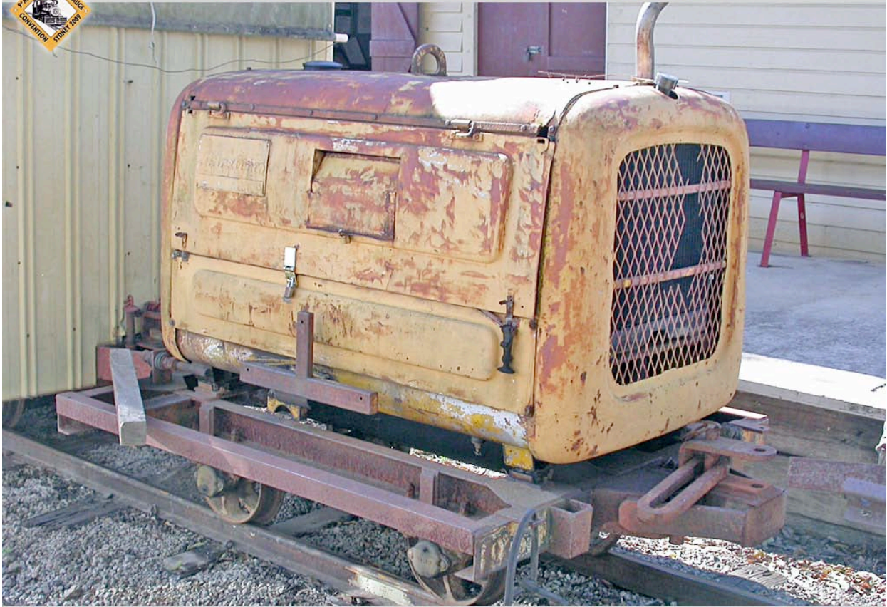
Ex-Moreton Mill, Atlas Copco compressor on wholestick frame, 2007
