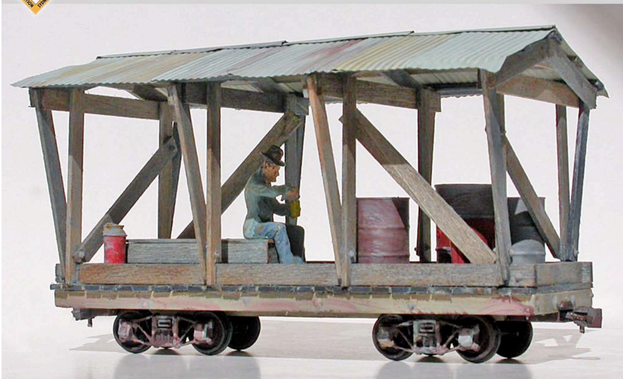
Scratchbuilt superstructure on Mountain Blue 18' 3" x 6' 4" On30 white metal underframe
