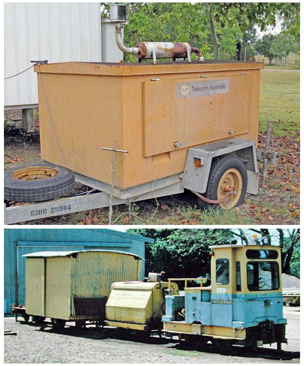
Here's a somewhat comparable mill-owned generator or compressor that appears to be mounted on an ex-cane bin underframe.
