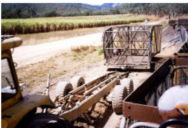
Winching bins onto a 2 bin trailer at a farm transfer point. Note the large timber bumper on the tractor (next column), which is used to move the bins while on the rails. Hitting the bins too hard is a frequent cause of bin damage.
