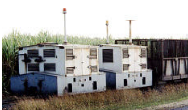
Mackay Sugar brake vans with flashing lights for visibility. Brake vans are essentially heavy weights with a small engine for powering the radio-controlled air brakes.
