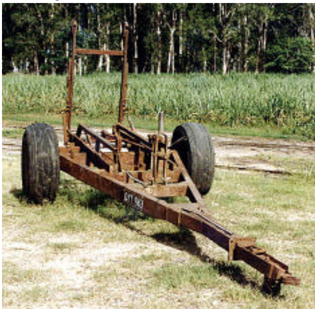
Single bin trailer with loading ramp so that a special rail transfer facilities are not required. This trailer's ramp drops over the rails and the bin is rolled directly onto the rails.
