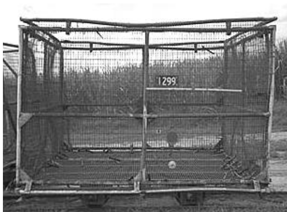
A older style 4 ton bin in rather sad repair. Note the extended top, welded corner braces and tubular frame.
