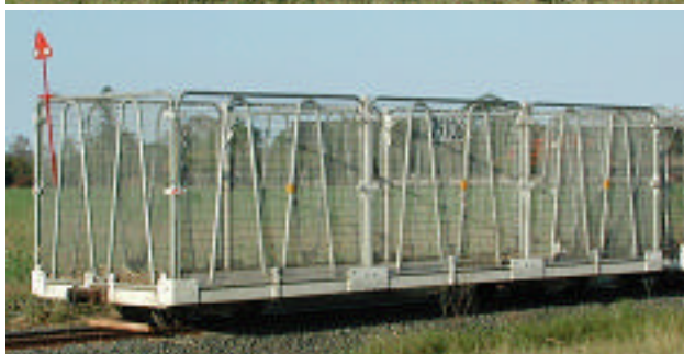
Pleystowe Mill's new extended bins, roughly ~15 ton load, on a well-graded main line leading to the mill. Note the concrete culvert under the upper bin.
