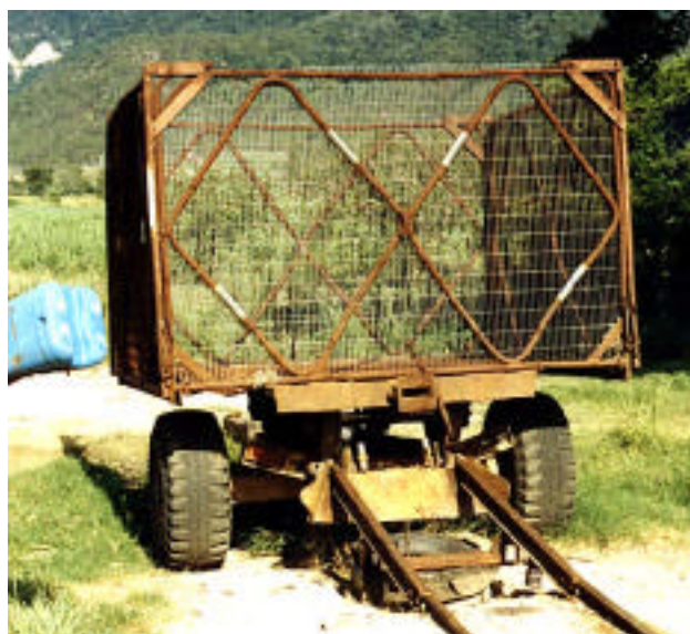
Single bin trailer with metal 'pan'. The trailer is backed into the ramp; the hinged rail ramp lifts so the bin can be transferred to/from the rails. Note the large metal springs near the hinge and the tire which prevents the ramp dropping too close to the ground for the guide pan.
