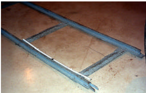
One half of a lightweight straight section with fastening yoke on nearest end. The white object is a metre measuring stick.
