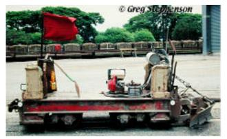
Ballast spreader for towing, but not likely heavy enough for pushing (above) and heavier unit (top next column). The CaneSIG web site has photos of several other designs. Try 'plough' or 'ballast spreader' (without the quotes) as search terms.
