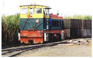
Mackay Sugar bogie locomotive, note the end-of-rake markers, jacks, lights, etc.
