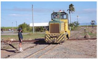
An off-sider holds the crossing as the cane loco crosses a lighter traffic QR line (above). Note the derail and signal
