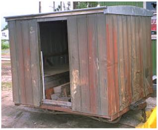
Looks like a garden shed: an aluminium sheathed tool shed on a cane bin chassis. The white object propped against the door frame is a metre stick.
