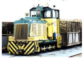
Mackay Sugar's Clyde-built Broadsound 0-6-0 loco. Note the end-of-rake markers, wooden chocks, fire extinguishers, air cleaner, horns, lights, etc.
