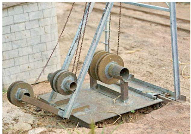
Working pulleys, L to R: Trolley back, load lift, & trolley out.
