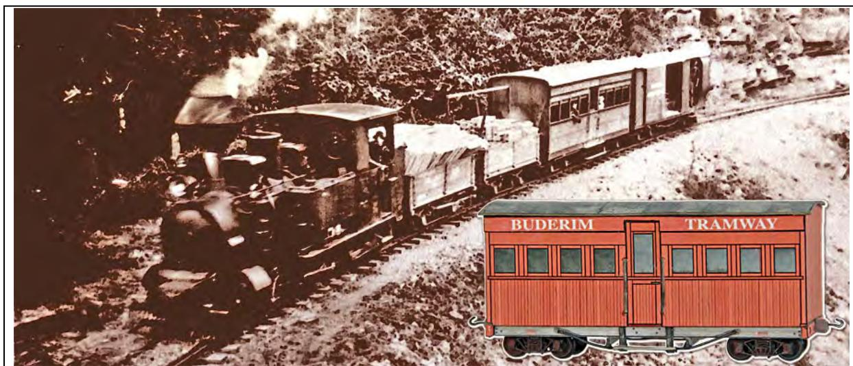
'Rounding the Curve, Buderim Mountain Queensland': the 30" gauge Krauss with a mixed goods and passenger train consisting of two 4w open wagons, the Buderim coach and the brake van. The inset shows a completed HOn30 photorealistic coach model (see NGDU #56 for details). The main image has been Photoshopped from a print in the Ted Ward Collection, photographer unknown.
