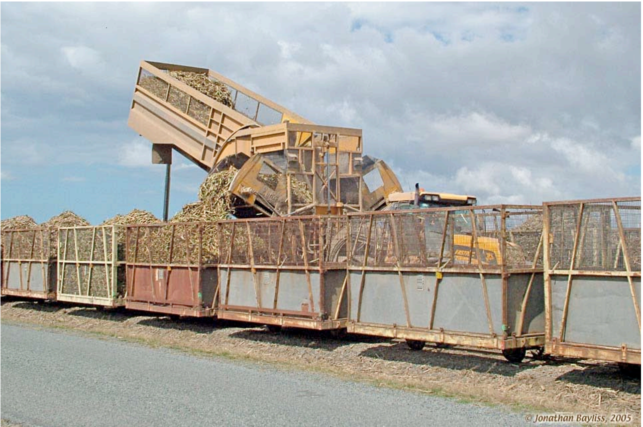
Tractor-pulled end-tipping, side-delivery, in-field transporter unloading at rail transfer point, Mackay area. 22 Aug 2005, Jonathan Bayliss photographer.
