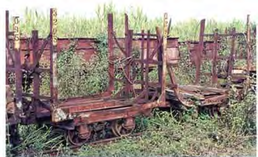
ABOVE: Steel wholestick cane trucks on the scrap line at Goondi Mill, 1982. The cradle on the left has been fabricated with braced uprights, while the one on the right has angle iron bent into a 'U' shape. Greg Stephenson photographer.
