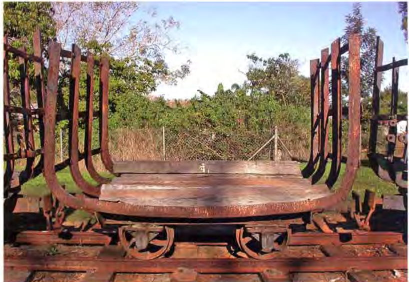
ABOVE: Lightweight steel cane trucks, Isis Mill, Huxley, 8 September 1968. The loops on the uprights would have been used for unloading and were unnecessary when mills shifted to grapples or rotary dumps. John Armstrong photographer.
