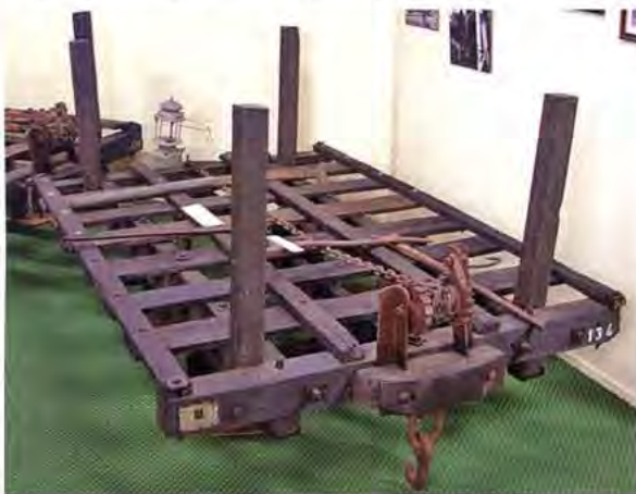
BELOW: Bundaberg Sugar wooden wholestick truck at Fairymead House, Bundaberg. The deck is open enough that it's fairly obvious this truck's structural integrity depends upon longitudinal, not diagonal, bracing. Lynn Zelmer photographer.
