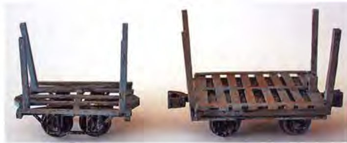
ABOVE: Scratchbuilt HO N 30 wholestick trucks using styrene strips. The steel truck (left) is built as close to scale as was possible when converting from 2' to 30" gauge and the use of commercial N scale wheelsets. The wooden truck (right) is more practical; it's built around a length of brass strip to provide strength and rigidity. The biggest modelling challenge is drilling and gluing the bearing blocks so that the wheelsets are square and at the same height.
