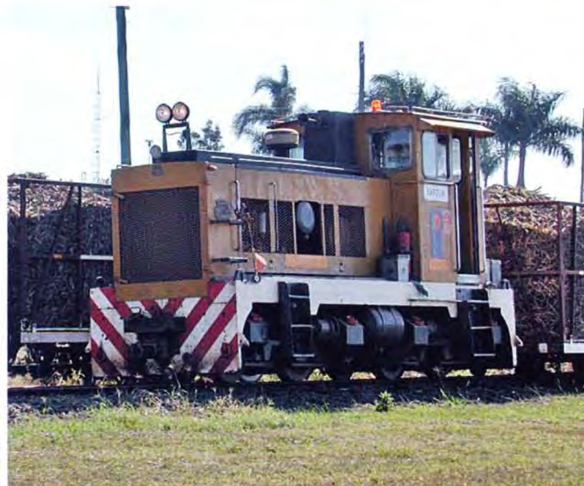
LEFT: Two shots of Millaquin Mill's Barolin, a 24 ton EM Baldwin locomotive (B-B DH 6456.1 11.75 of 1975, DH24B Mk6). Note that aside from the curves of the cab and bonnet roofs the locomotive is quite 'boxy', with flat and relatively plain surfaces, making for easy modelling in brass or styrene. Lynn Zelmer photographer.
