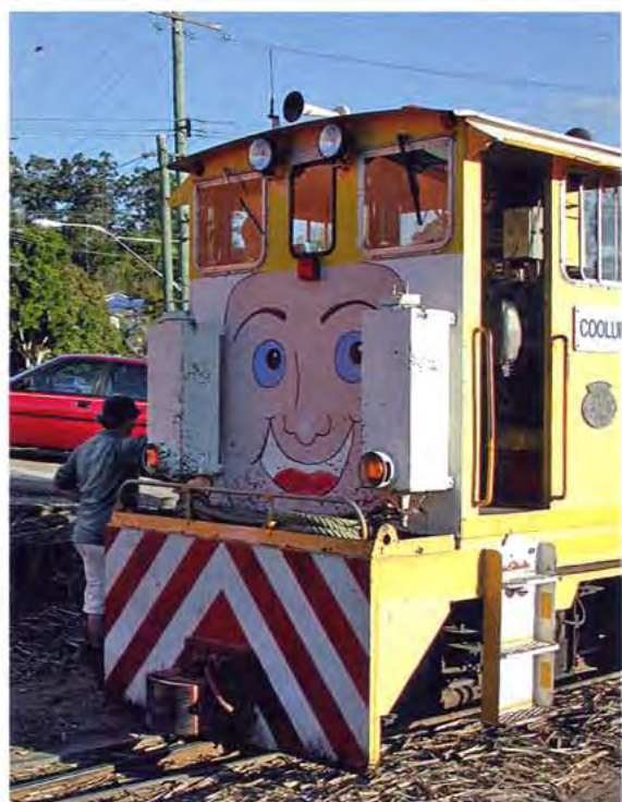
ABOVE: Lorry's 'Clickety Clack - Stay Clear of my Track' message was the centrepiece of Moreton Mill's public safety program and a favourite of Nambour kids for several years before the Mill's closure (Coolum, EM Baldwin B-B DH of 1974). The message was especially important as the Nambour Mill track ran down the middle of one of Nambour's busiest city centre roads. Lynn Zelmer photographer.
