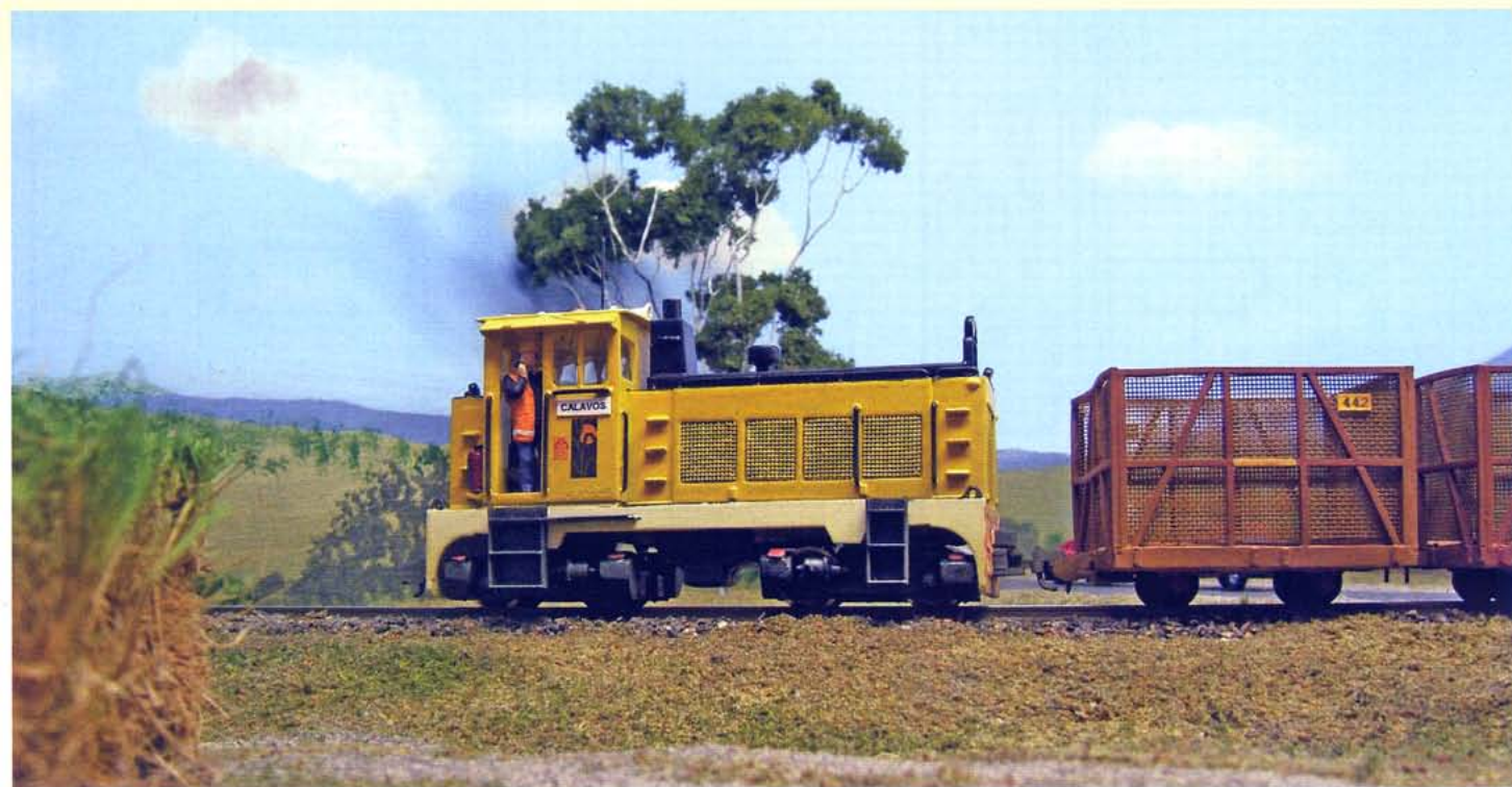
BELOW: Lincoln Driver's HOn30 model of Oakwood (Bingera Mill, EM Baldwin B-B DH 5800.1 5.75 of 1975, DH26B Mk2) operating on his Wallaville exhibition layout. Bingera operated this locomotive with Locotrol master/slave controls. John Dennis photographer.
