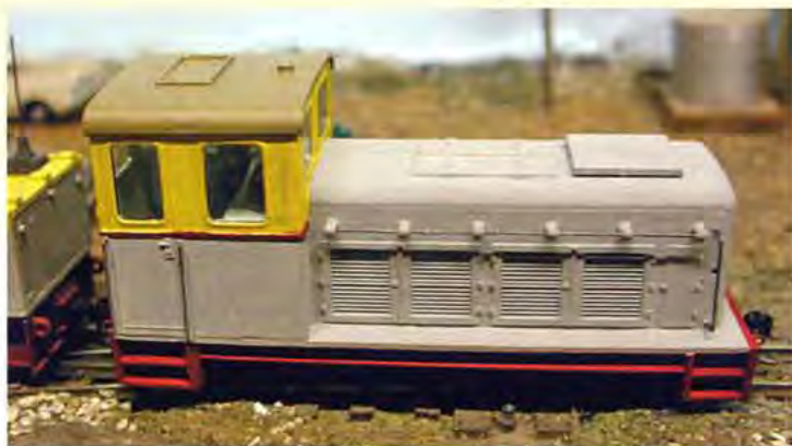
ABOVE: Greg Stephenson's HOn30 B-B DH cane locomotive from UK Knightwing OO scale 0-4-0 standard gauge kit modified to fit an N scale Lifelike B-B diesel mechanism. Lynn Zelmer photographer.
