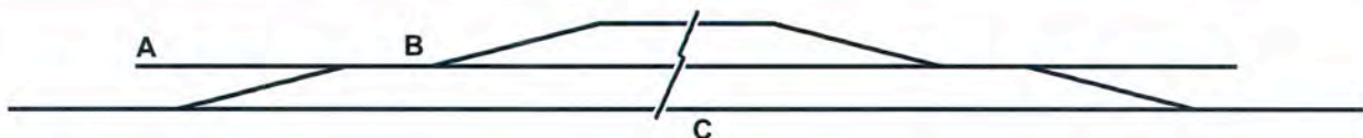
A simple farm siding, perhaps 500 metres long in level country. The loaded bin ramp (A) is roughly 450 mm above the through road (C), the storage tracks (starting at B) are roughly 300 mm above the through road with the elevation falling slightly to the empty bin pickup point at the right of the siding (see photo of haul over pickup point). The through road is ballasted with gravel and is separated from the shire maintained gravel or bitumen road which parallels it by a shallow ditch. Other tracks are trash covered, with standing water in the wet season.
