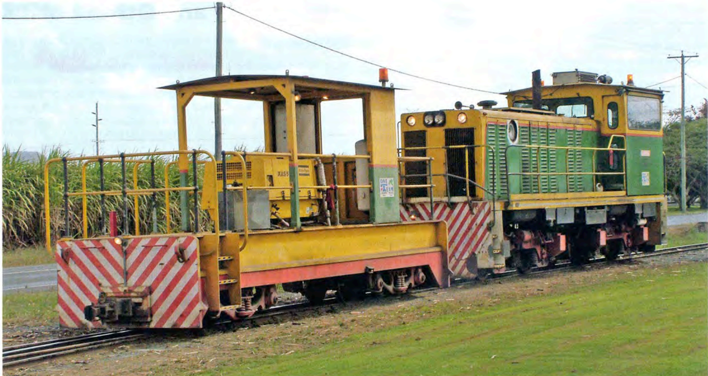
ABOVE: Even bogie locomotives need extra help with large rakes of cane. Here is Mackay Sugar's B-B DH loco #55 Balbera (Walkers 657 of 1970, rebuilt TulkGon 1994) running light with a bogie brake van, 25 August 2005. Jonathan Bayliss photographer.
