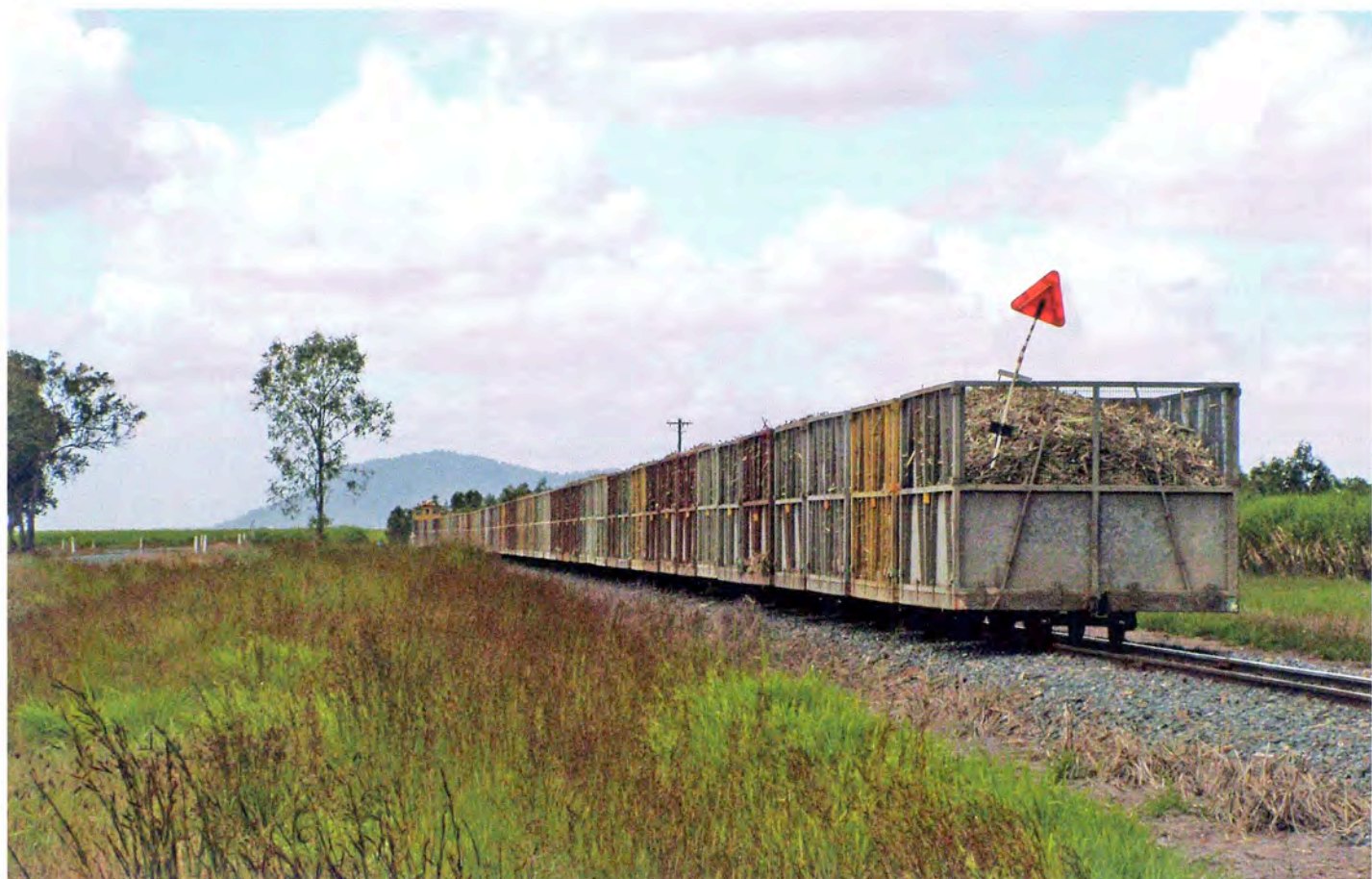
BELOW: End-of-rake markers come in a variety of styles, this triangular end-of-rake marker is on a rake of full bins, likely behind Mackay Sugar's 0-6-0 DH #54 Oakenden (Com-Eng FB3169 of 1963), 25 August 2005. Jonathan Bayliss photographer
