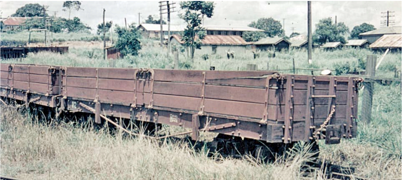
Innisfail Tramway “H” wagon used for carting bagged sugar from South Johnstone and Mourilyan Mills to Mourilyan Harbour. D Sheehan, photographer.
