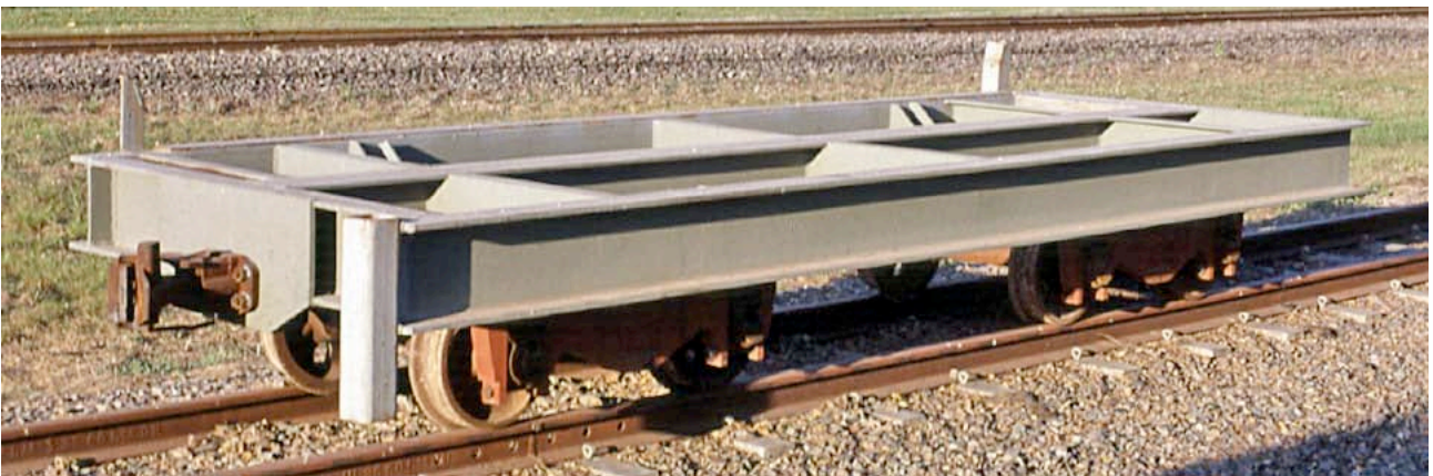
New bulk sugar wagon underframe at Victoria Mill in 2000. Greg Stephenson, photographer.
