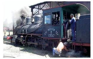
Although more tourists are visiting the mills to view and ride on the trains, their main purpose is to haul sugar cane from the 'acopio' (loading point) to the mill. Thus many of the locos are thrashed about with full loads; there is lots of slipping and sliding, and hand sanding to get the trains moving, and a lot of black smoke from the low grade of oil burned. It all makes for a great
