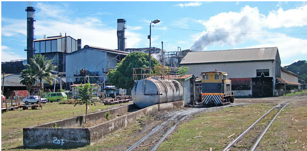
Baldwin #16 being refueled at the Lautoka Mill, 2007. The loco shed is the relatively new building on the right. Note the long narrow containment barrier around the fuel tanks, it's located between two parallel tracks and presumably needs the length for sufficient capacity in case of a spill. Lynn Zelmer, photographer.
