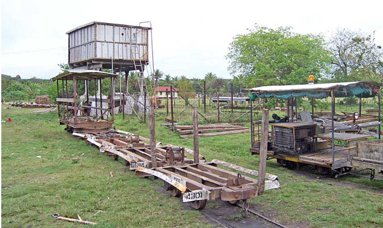
Cuvu depot on the southern part of the Lautoka Mill network. Linecar 6 (probably of Wickham ancestry), with empty cane trucks and a labour truck parked on one leg of the turning triangle. The large water tank was a necessity in steam days. 5 October 2006. John Browning, photographer.
