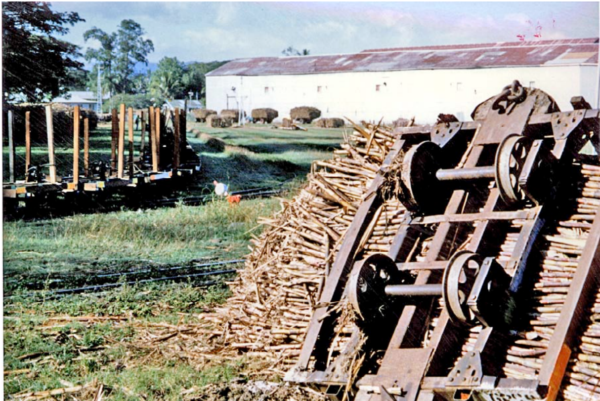
Derailed wholestick trucks are common, this one shows the underframe construction and the square wheel bearing blocks. Lautoka, 1988. Ross Evans, photographer.
