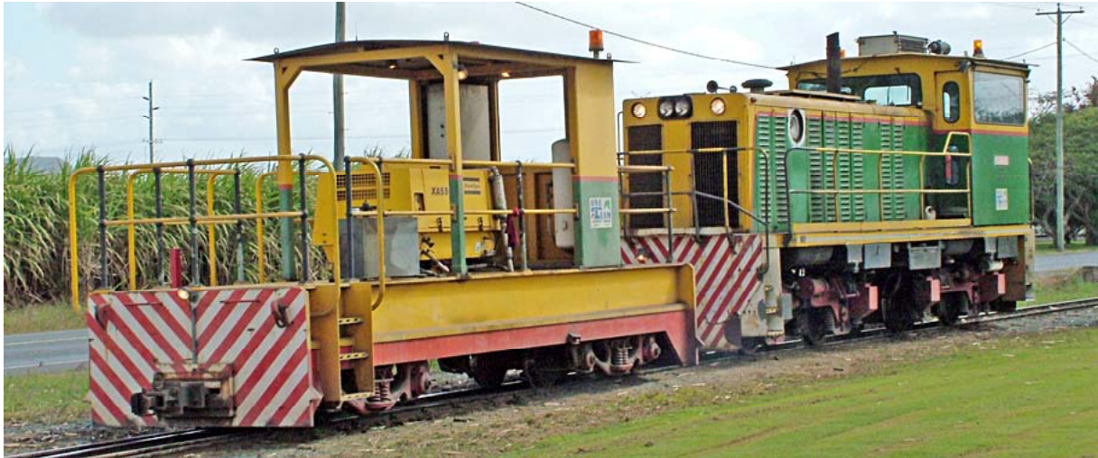
Mackay Sugar B-B DH loco #55 Balberra (Walkers 657 of 1970, rebuilt TulkGon 1994) with bogie brake van. 25 Aug 2005. Jonathan Bayliss photographer.
