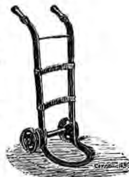
Fig. 3186. Bay-Barrow. Capacity 150 and 200 kilos.
