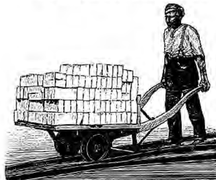
Fig. 3178. Track Barrow to carry 600 to 750 kilos burned bricks. Gauge 500 mm.
