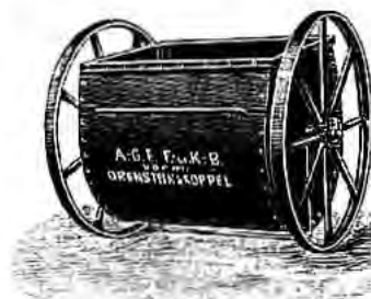
Fig. 3183. Tipping Barrow to carry malt and grain. Tips round the axle. Standard Sizes: 200, 800 and 400 lbs. capacity.
