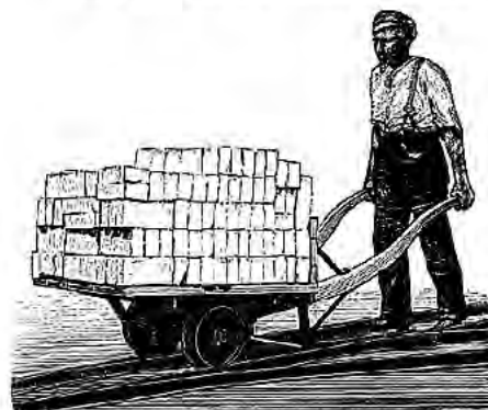
Fig. 3178. Track Barrow to carry 600 to 750 kilos burned bricks. Gauge 500 mm.
