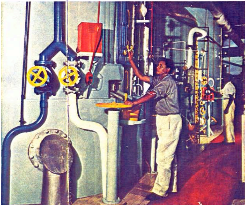
BELOW: Large vessels at Rarawai mill in which cleaned juice crushed from sugar cane is boiled until sugar crystals form.
