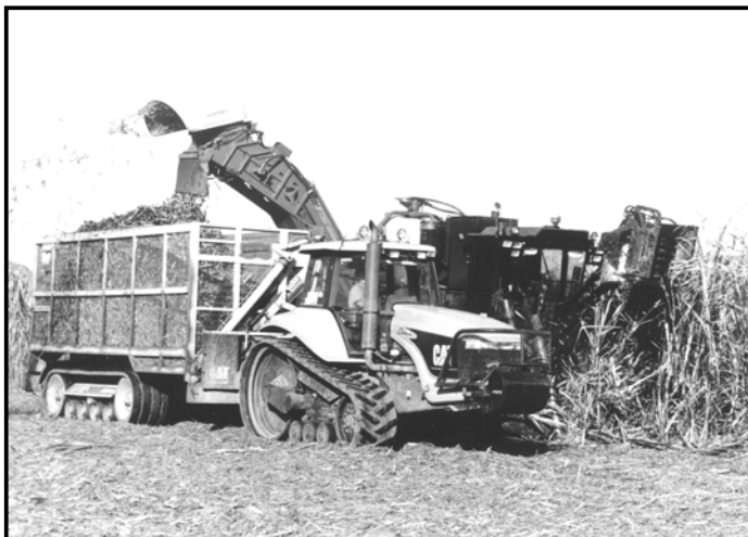
2000 This mechanical harvester working on Quirk's farm near Stotts Island cuts 100 tonne per hour. Photo Louise Devine
