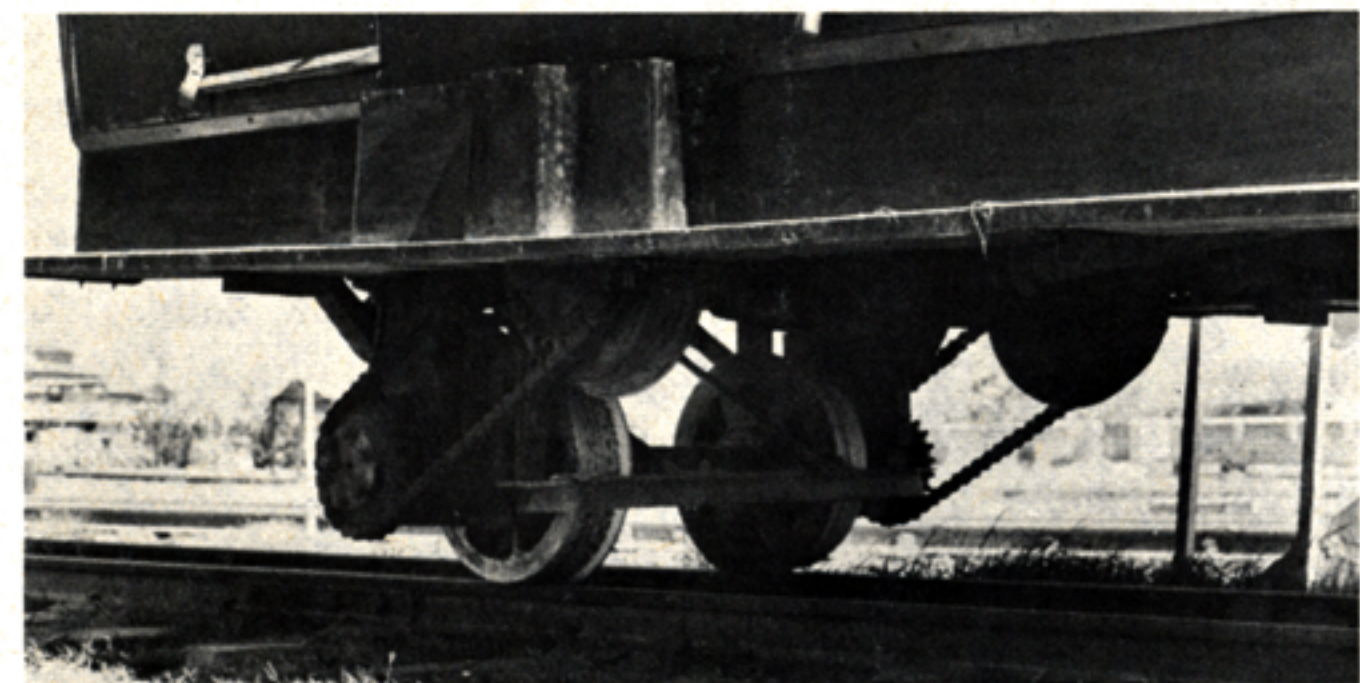
Railmotor KS12 of the Kalka-Simla Railway, built by Wicham & Co. of Ware, England, in 1931, seats four on inspection duty, last used in 1967, 58 BHP motor, 2'6" gauge.
