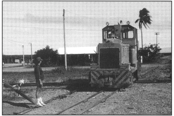
A Clyde-built diesel hydraulic locomotive crossing the government line at Racecourse Mill near Mackay in 1990. There were eight such locomotives working up to 40 kilometers from the mill. Each had a two-man crew, radio contact with the dispatcher, and had to set derails whenever they crossed the main QR line.
