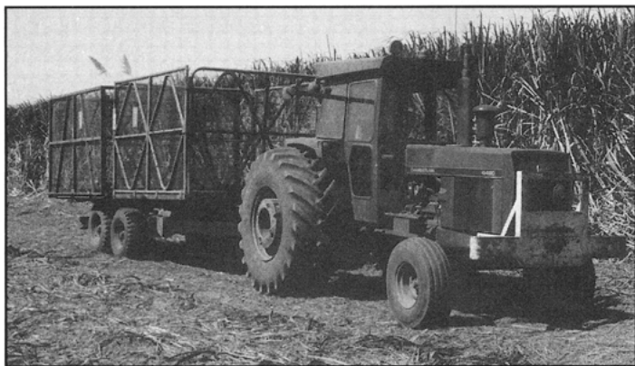
Two empty standard chopped cane cars on one type of tractor-pulled trailer. The cars are 'railed' onto the trailer with a winch and can easily be rerailed back onto the track for collection.
