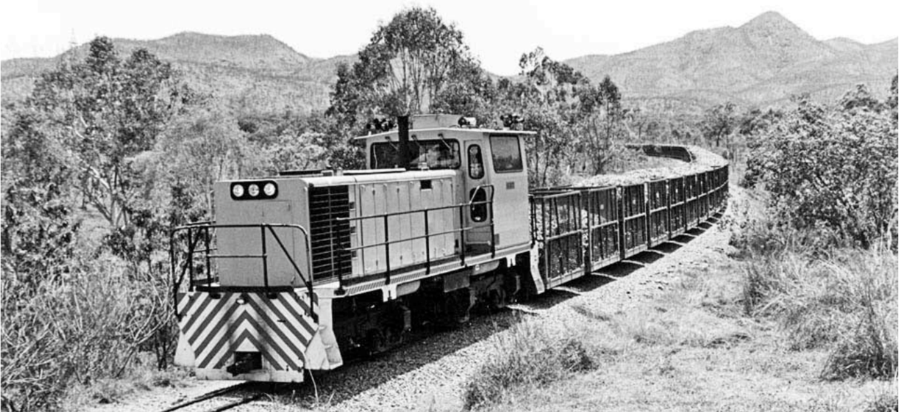
Invicta Sugar Mill's Scott (B-B DH, rebuilt 1995) brings back the last cane from the Dalbeg area for the 1999 season. The locomotive was converted from 1435mm gauge in 1995 when rebuilt from ex-State Rail Authority of New South Wales 7310 of 1971. Carl Millington, photographer.
