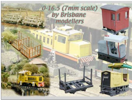
A selection of mostly scratchbuilt O-16.5 locos and rollingstock built by Brisbane modellers using a variety of construction materials including brass, styrene and resin-molded components.
