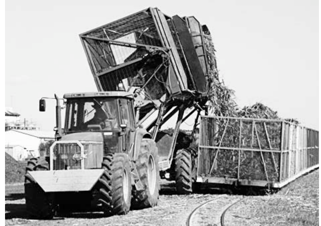
The front compartment of the two compartment tractor-hauled infield transporter (right) has already been emptied and is descending back into place. The rear compartment is still being elevated and will tip far enough to completely empty. Lynn Zelmer, photographer.
