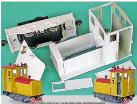
Comeng Model A inspired On30 4w DM locomotive, scratchbuilt styrene superstructure on a Boulder Valley resin chassis, power unit from a HO Bachmann 44 ton diesel and Circuitron flashing light. The white pole and sign on the rear of the loco is an end-of-rake marker.
