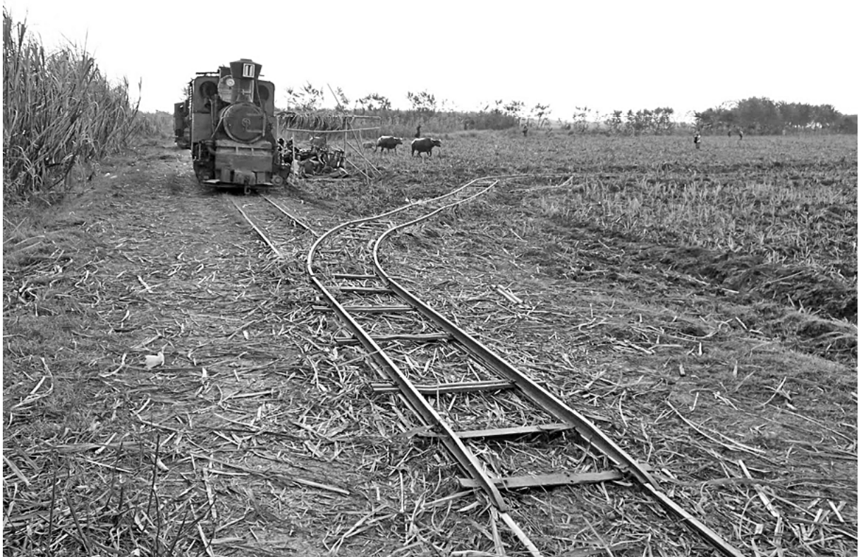
Java: Sumberharjo is one of the few mills left in Indonesia to operate field lines. The area is low-lying and obviously flood-prone, with extensive drainage works having built through what were once swamps, so the future of these tramways is quite optimistic. Here domestic water buffalo haul cane trucks over temporary track laid in the fields. John Browning photographer, July 2010.
