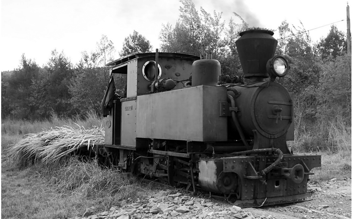
South Africa: Douth African Railways branch, Umtwalume Valley Estates #2, a 2' gauge still working Avonside built in 1933. John Browning photographer, June 2010.
