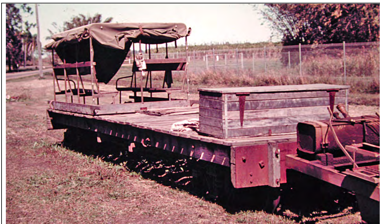
Fairymead Mill navy bogie flat wagon with canvas covered enclosure with benches, tool box and space for additional tools and supplies, 1981. Greg Stephenson photographer.
