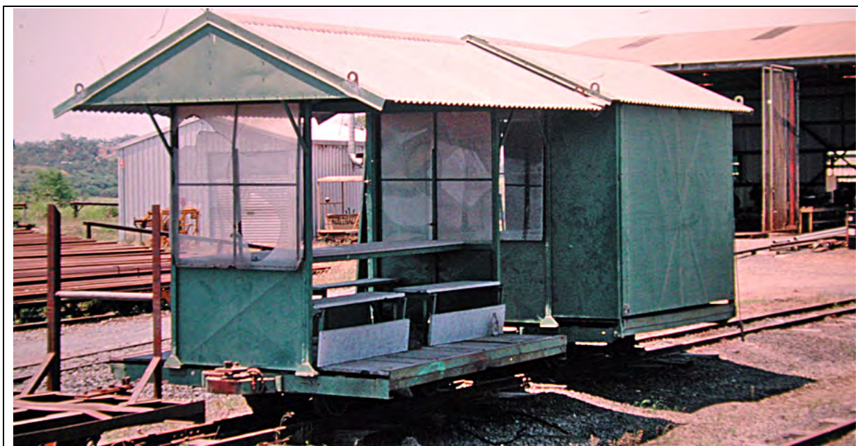
Farleigh Mill, Navy Transport and storage on cane bin underframes, 18 October 1997. Note the use of modern 'shed' materials and the lifting rings on the roofs. Greg Stephenson, photographer.
