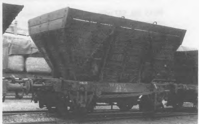
VR15687 is different from the VR on the left - the additional boards on the side of the hopper are canted and a second set of lifting lugs added. The lifting lugs allowed overhead cranes to lift the body off the underframe for discharge of coal into large stockpiles, such as into the hold of a ship. (late S. Suggit)
