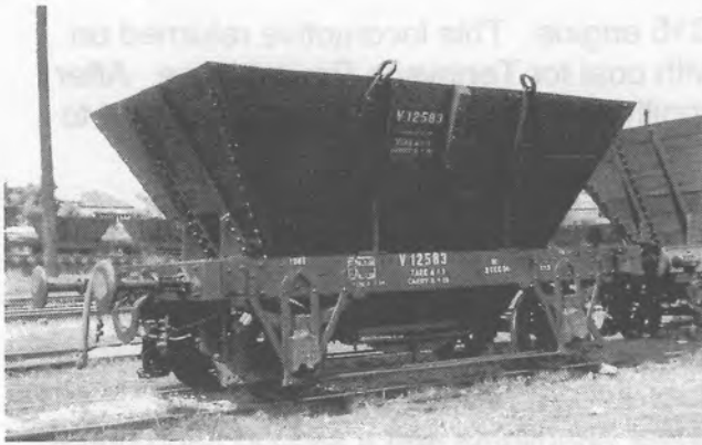
The standard Queensland coal hopper - the V class. There were several variants of this classification. The major differences were in the dimensions of the hopper body, some being longer and/or higher than others. (late S. Suggit)
