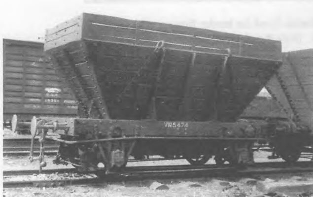
A number of V wagons were altered, being fitted with additional boards to increase capacity and reclassified VR. The boards on VR5474 are vertical all around. (late S. Suggit)
