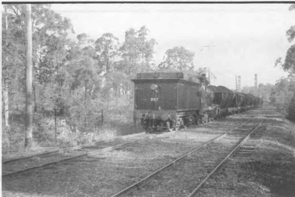
PB15 No. 587 with rear headlight and twin sand domes fitted for tender first running works a string of loaded hoppers on the New Chum Branch. Note the absence of a van.
