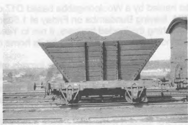
A VJ class hopper with timber underframe and body. This was the most common form of VJ. Forty of these hoppers were altered, fitted with lifting hooks and reclassified VJM.
