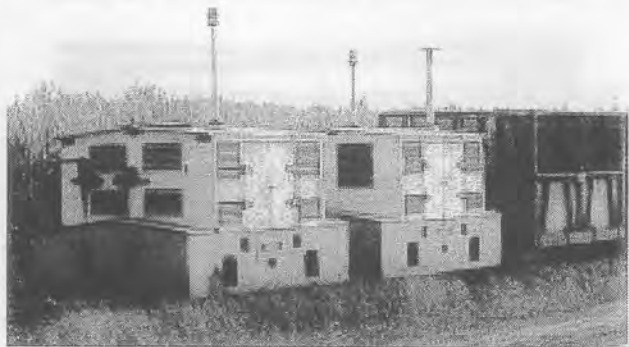
Mackay Sugar brake vans with flashing lights for visibility. Brake vans are essentially heavy weights with a small engine for powering the radio-controlled brakes.
