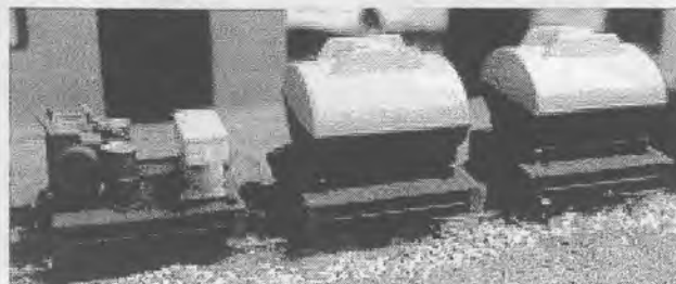
Inspired by a weed spraying train seen at Bingera Mill, Greg Stephenson fitted tanks from a Hasagawa 1:72 refuelling tanker to 4 wheel underframes (above).
