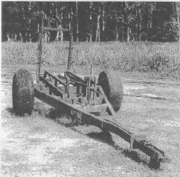
Single bin trailer with loading ramp so that a special rail transfer facilities are not required. The trailer's ramp drops over the rails and the bin is rolled directly onto the rails.
