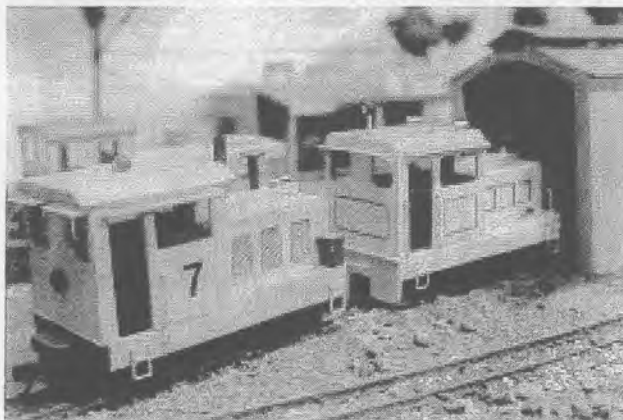
Two HOn30 freelanced cane locos built from Bob Dow's plans and notes ( http://www.ozemail.com/~ozbob ). Built from styrene, they use Bachmann N gauge mechanisms, and are sitting in front of Bob's Dowmont cane field-style engine shed.
