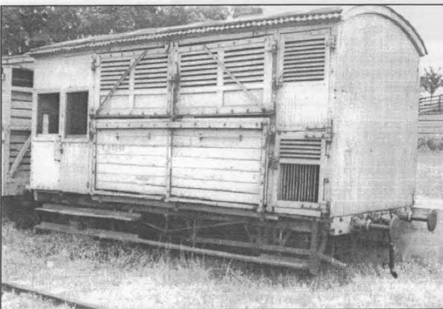
Two images of a Z class four wheel horse box. An attendant's compartment is at one end, with a dog box at the other.
