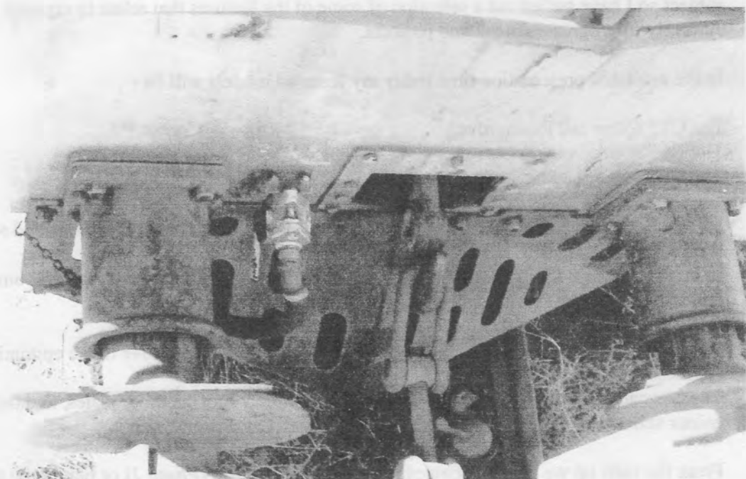
Photo 2 – Plate Steel Cowcatcher
