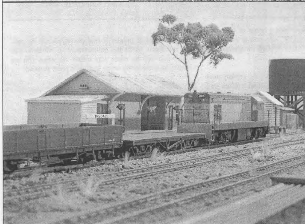
Another view of Iredale which clearly shows the chaired rail. Note the lack of shouldered ballast in the sidings, this was not an unusual feature. In the foreground is the fetters rail rack.
