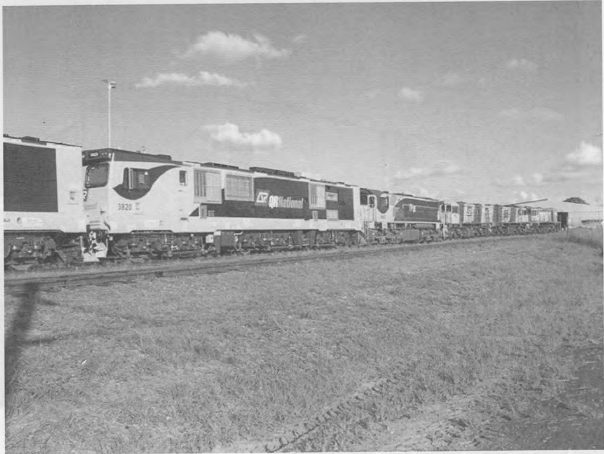
Locomotive shunt arriving at Acacia Ridge from Fisherman Islands. 2 x 3800 EL, 2470 Class, and 3 x 1720 Class Locomotives in three different liveries.
