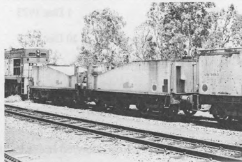
QR LTM wagons – converted from steam locomotive tenders [Image : Brian Webber – “waste not, want not”]
